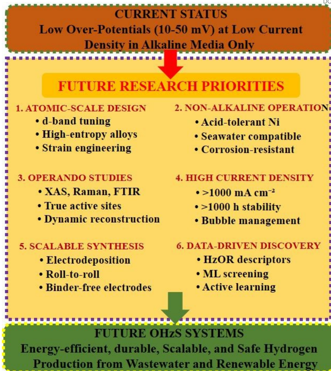
Fig 12. Schematic roadmap for future directions in Ni-based electrocatalysts for hydrazine-assisted hydrogen production (OH 2 S).
