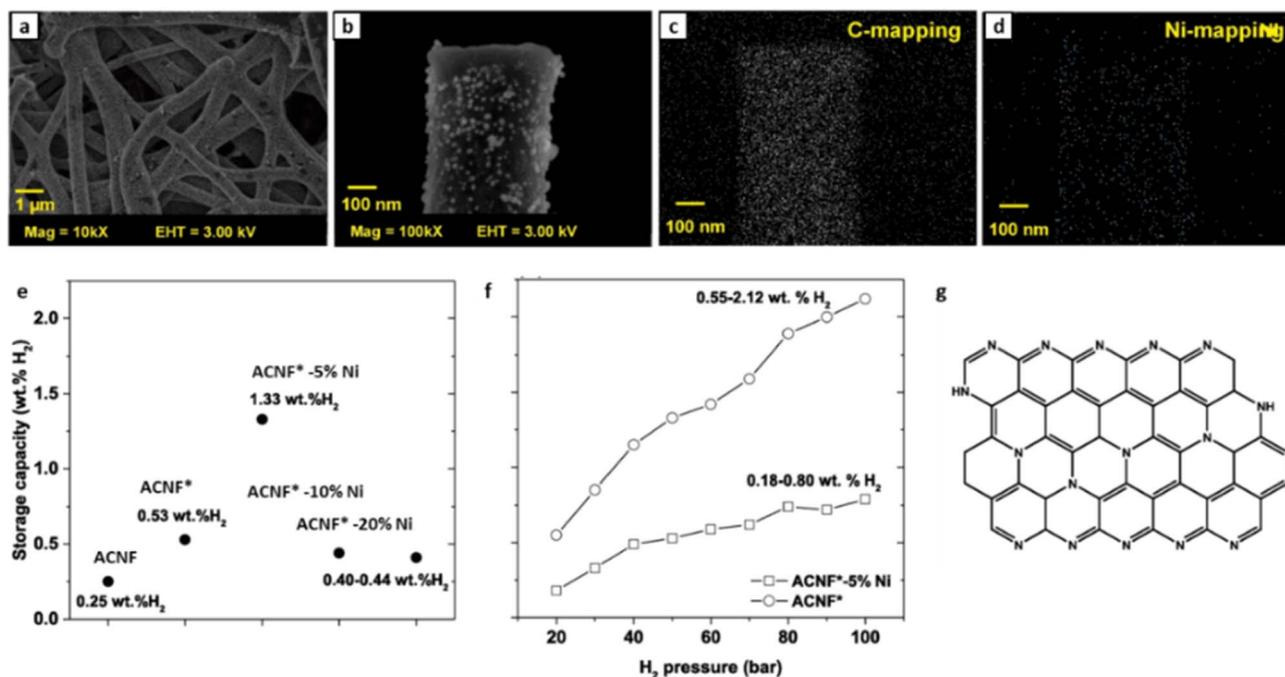
Fig. 6 Improving the H<sub>2</sub> adsorption of activated carbons via metallic nanoparticle decoration. (a–d) SEM images and EDX-mappings of 5 wt% Ni-doped ACNFs, (e and f) H<sub>2</sub> adsorptions at RT of ACNFs with and without Ni-doping with different Ni content, and (g) chemical structure of ACNF<sup>67</sup> (reproduced from ref. 67 with permission from Elsevier, copyright 2021).
