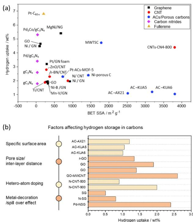
Fig. 7 (a) Comparison of the H<sub>2</sub> storage capacities of carbon-based adsorbents with respect to their specific surface area and (b) factors affecting the hydrogen storage in carbon-based materials.
