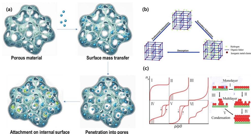
Fig. 2 (a) Illustration of the mechanism of hydrogen adsorption in porous materials, (b) hydrogen storage mechanism in MOFs<sup>36</sup> (reproduced from ref. 36 with permission from Elsevier, copyright 2024), and (c) different types of adsorption isotherms<sup>37</sup> (reproduced from ref. 37 with permission from Scientific Research, copyright (open access) 2018).
