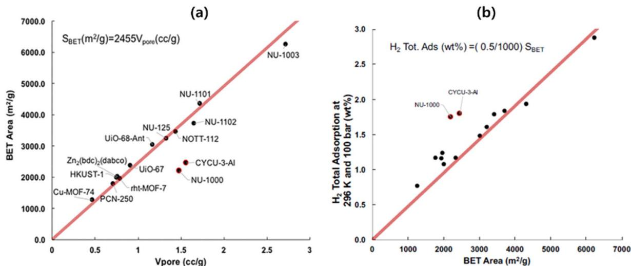
Fig. 8 Comparison of (a) BET surface area and pore volume, and (b) total H<sub>2</sub> uptake with respect to the BET surface area<sup>52</sup> (reproduced from ref. 52 with permission from The American Chemical Society, copyright 2018).
