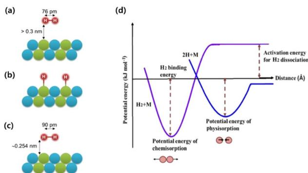
Fig. 1 (a) Physisorption, (b) chemisorption, (c) weakly bonded hydrogen,<sup>29</sup> (reproduced from ref. 29 with permission from Wiley, copyright 2015), and (d) one-dimensional potential energy profiles for physisorption and chemisorption processes plotted as a function of the separation distance between H<sub>2</sub> molecules and the substrate. Reprinted with permission,<sup>25</sup> (reproduced from ref. 25 with permission from Wiley, copyright 2025).
