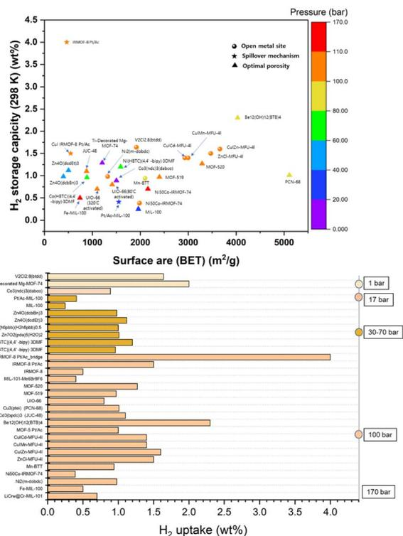
Fig. 11 Comparison of the H<sub>2</sub> storage capacities of different types of MOFs concerning surface area and pressure at RT.
