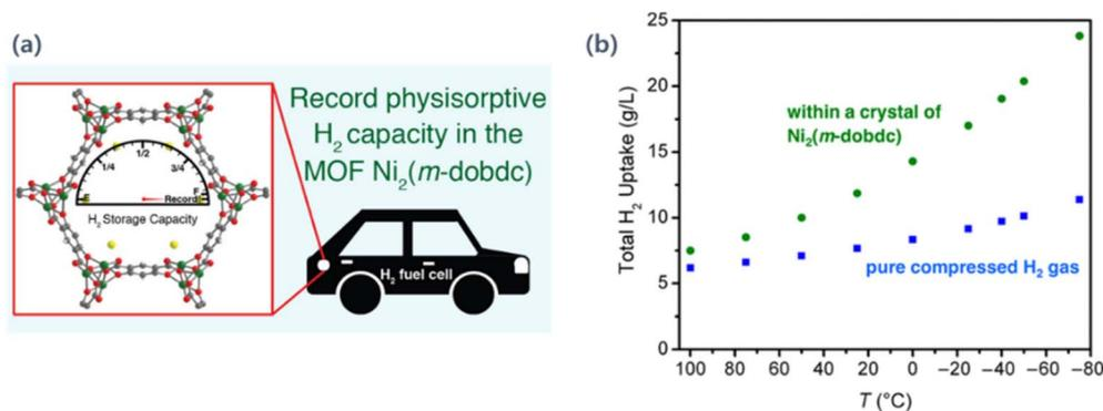
Fig. 9 (a) Schematic illustration of the physisorptive H<sub>2</sub> capacity in Ni<sub>2</sub>(*m*-dobdc) and (b) comparison of total volumetric capacities and pure compressed H<sub>2</sub> of Ni<sub>2</sub>(*m*-dobdc) at 100 bar<sup>147</sup> (reproduced from ref. 147 with permission from The American Chemical Society, copyright 2018).
