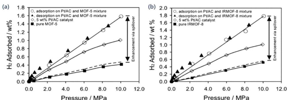
Fig. 10 Comparison of H<sub>2</sub> storage isotherms showing enhancement *via* the spillover effect for (a) pure MOF-5 and modified with Pt/Ac and (b) IRMOF-8 modified with Pt/Ac at 298 K<sup>150</sup> (reproduced from ref. 150 with permission from The American Chemical Society, copyright 2006).
