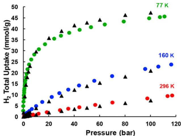
Fig. 4 Experimental (circles) and simulated (triangles) total hydrogen adsorption isotherms at 77 K (green), 160 K (blue), and 296 K (red) for NU-125<sup>52</sup> (reproduced from ref. 52 with permission from The American Chemical Society, copyright 2018).
