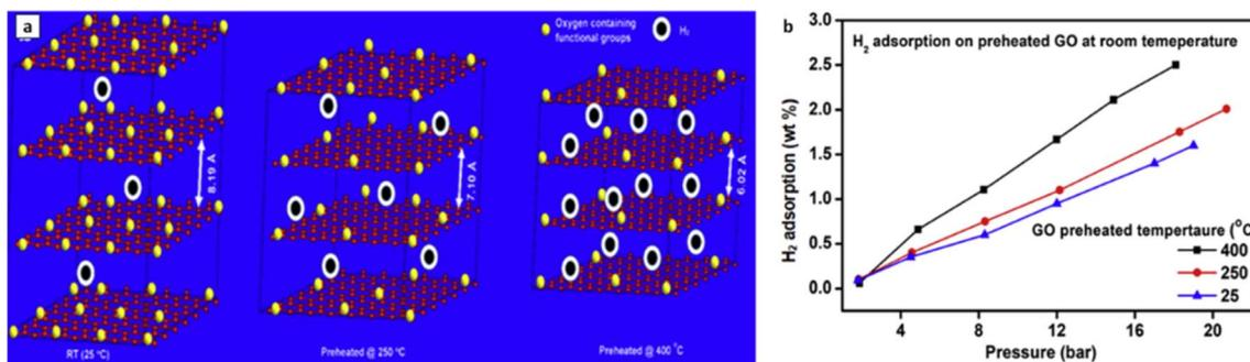
Fig. 5 The effect of interlayer distance of GO on H<sub>2</sub> adsorption (a) the control of interlayer spacing by altering the pretreatment temperature, (b) the H<sub>2</sub> adsorption properties of GO samples with different interlayer distances<sup>77</sup> (reproduced from ref. 77 with permission from Elsevier, copyright 2020).
