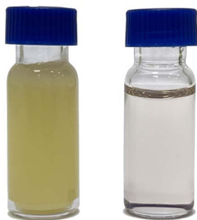
Fig. 5 Image of raw, untreated lipid feedstock (left) and hydrotreated lipid oil (right), highlighting the increase in clarity.
