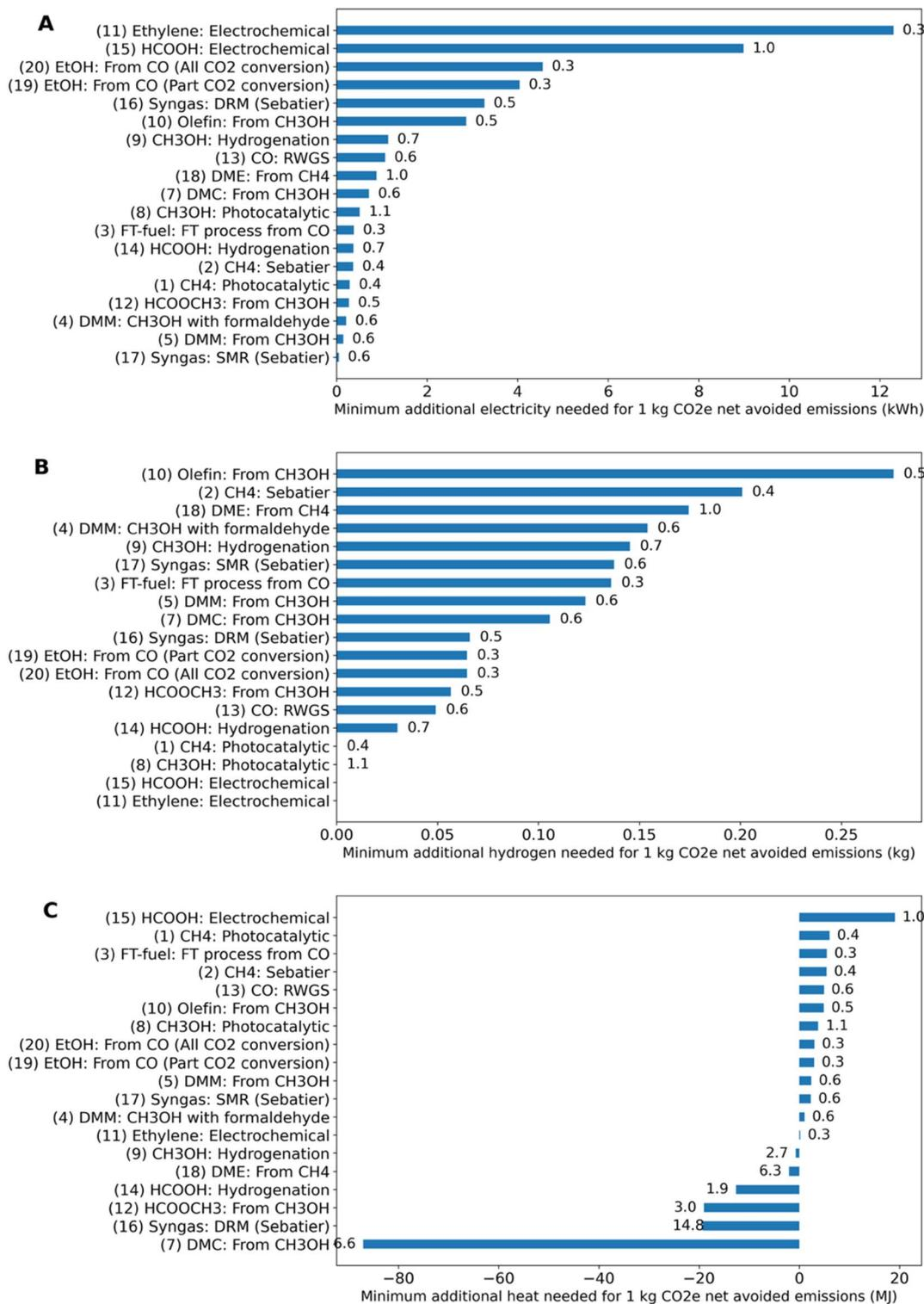
Fig. 5 Minimum additional demands for electricity (A), hydrogen (B), and heat (C) for 1 kg CO<sub>2</sub>e of net avoided emissions for each of the CCU pathways from across the 2050 background system scenarios. The numbers beside the bar show the quantity (in kg) of the corresponding final product required. In subplot B, pathways 11 and 15 do not require hydrogen as a feedstock in incumbent or CCU pathways, so there is no effect on hydrogen demand.
