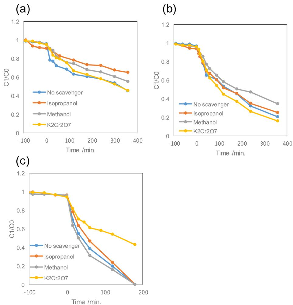
Fig. 4 The glyphosate degradation study of BiOBr with different facets: (a) (001), (b) (010), and (c) (102), respectively. The scavenger reagents were added at time zero. Isopropanol, methanol, and  $K_2Cr_2O_7$  are used as scavengers for OH radicals, holes, electrons, and superoxide anions, respectively.
