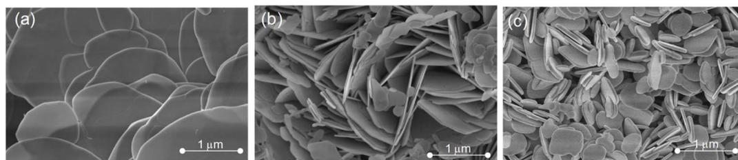
Fig. 2 SEM images of BiOBr with dominant facets: (a) (001), (b) (010) and (c) (102).
