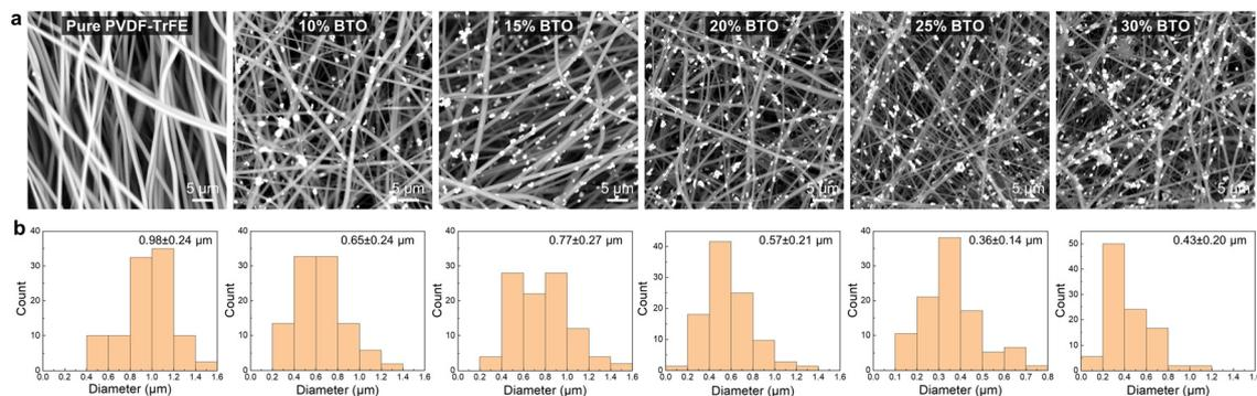
**Fig. 2** SEM images (a) and corresponding fiber diameter statistics (b) of pure PVDF-TrFE nanofibers and PVDF-TrFE/BTO composite nanofibers with a BTO content of 10, 15, 20, 25, and 30%, respectively.
