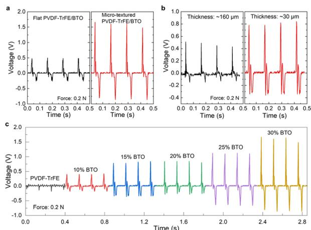
**Fig. 5** (a) Comparison of output voltage from piezoelectric pressure sensors made from the flat and micro-textured PVDF-TrFE/BTO (30%) nanofiber mat. (b) Comparison of output voltage from piezoelectric pressure sensors made from micro-textured PVDF-TrFE/BTO (20%) with different thicknesses (160 and 30  $\mu\text{m}$ ). (c) Typical output voltage of piezoelectric pressure sensors made from the micro-textured PVDF-TrFE/BTO nanofiber mat with different BTO contents.
