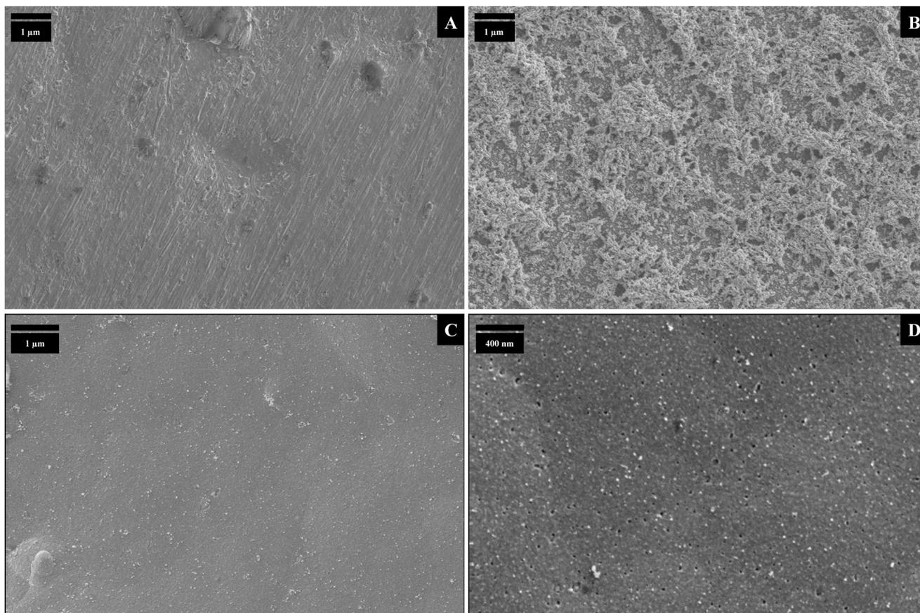
**Fig. 3** Surface characterization: scanning electron micrographs (SEM). A) SEM image of planar gold. B) SEM image of a highly porous gold electrode. C) SEM images of the molecularly imprinted polymer (MIP) on planar gold electrodes. D) SEM image of the molecularly imprinted polymer on HPG electrodes.
