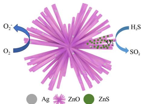
Fig. 9 Schematic diagram of the sensitivity mechanism of the Ag/ZnO sensor to H<sub>2</sub>S gas at 92 °C.
