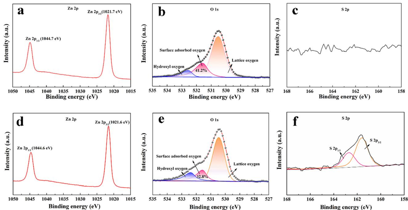
Fig. 8 The XPS spectra of Zn 2p, Ag 3d and O 1s of 3 at% Ag/ZnO composites (a–c) before and (d–f) after exposure to H<sub>2</sub>S gas at 92 °C.
