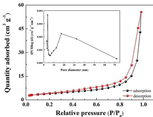
**Fig. 3**  $N_2$  adsorption–desorption curve and pore size distribution (inset) of Ag/ZnO composites with a molar ratio of 3 at% Ag.
