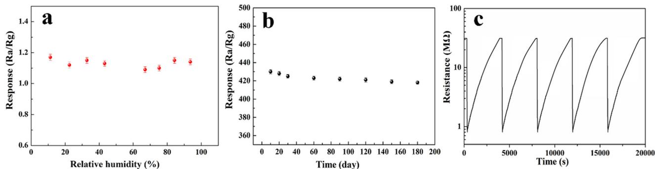
Fig. 7 Response of the 3 at% Ag/ZnO sensor at 92 °C: (a) the responses in different relative humidity atmosphere, (b) long-term stability to H<sub>2</sub>S, (c) repeatability to 10 ppm H<sub>2</sub>S.
