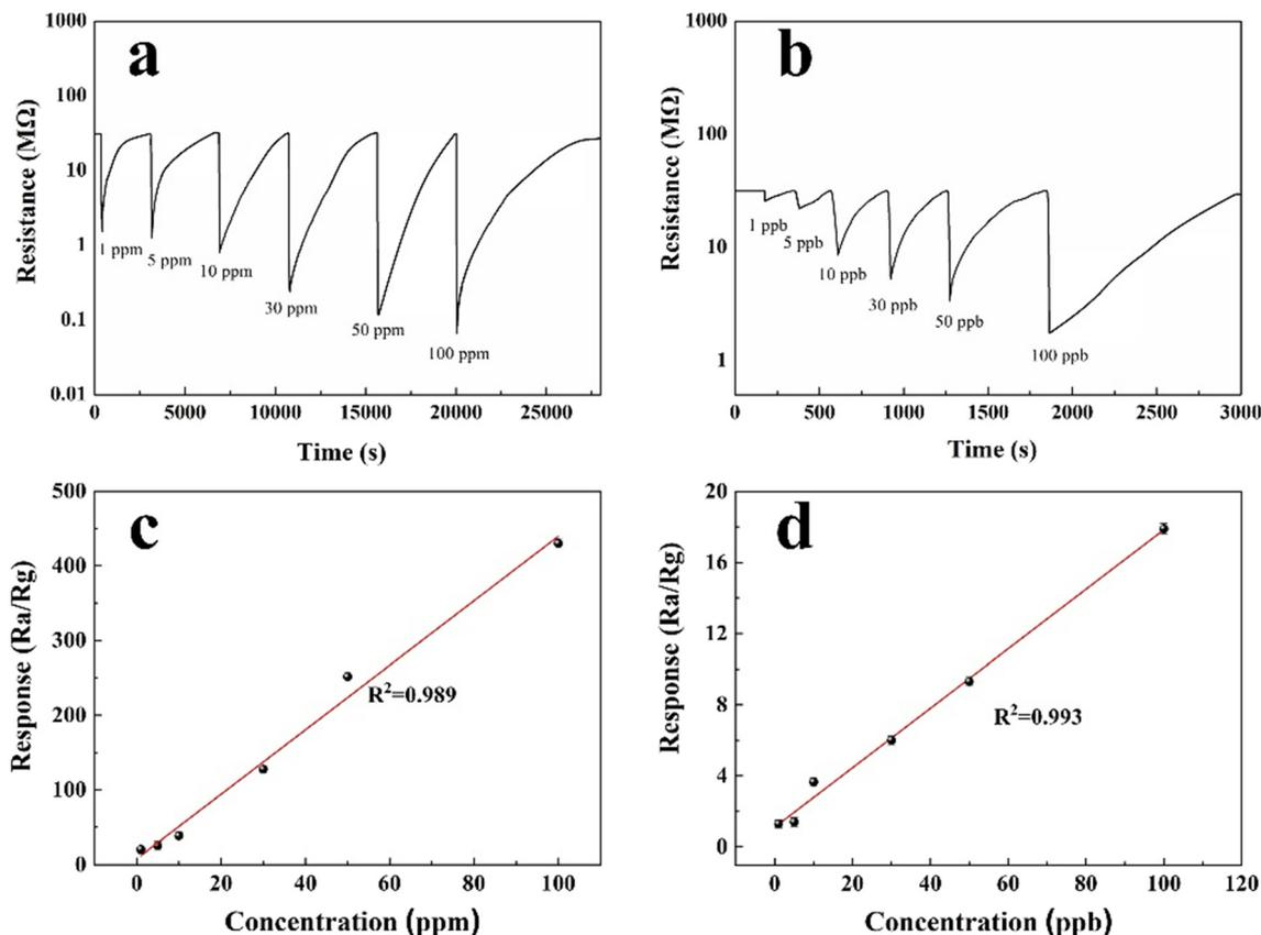
Fig. 6 Ag/ZnO sensor with 3 at% Ag load molar ratio at 92 °C: (a) response recovery curve and (c) linear relationship for 1–100 ppm H<sub>2</sub>S gas, (b) response recovery curve and (d) linear relationship for 1–100 ppb H<sub>2</sub>S gas.
