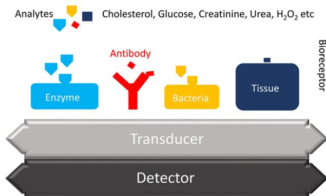
Fig. 1 A visual representation of a biosensor.
