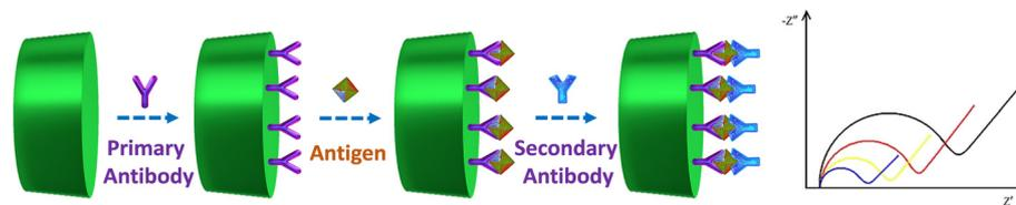
Fig. 5 Schematic representation of an impedimetric biosensor.
