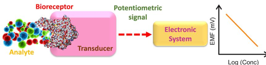
Fig. 2 Diagrammatic representation of the potentiometric biosensor.
