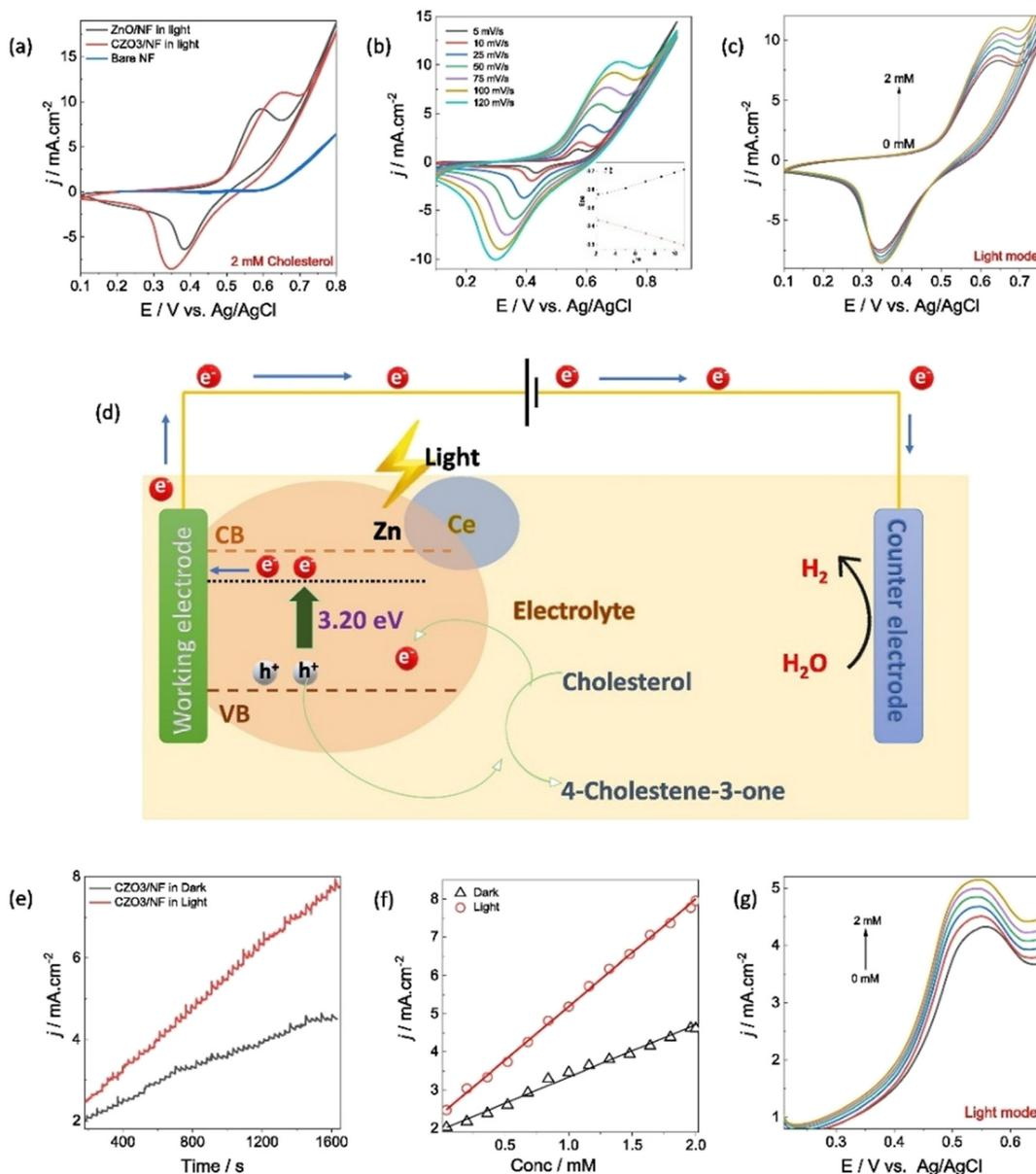
**Fig. 8** The study involving (a–c) CV, (e and f) chronoamperometry, and (g) DPV, along with the proposed (d) mechanism of cholesterol oxidation in photoelectrochemical cholesterol biosensors (reprinted from ref. 113 with permission from Elsevier).
