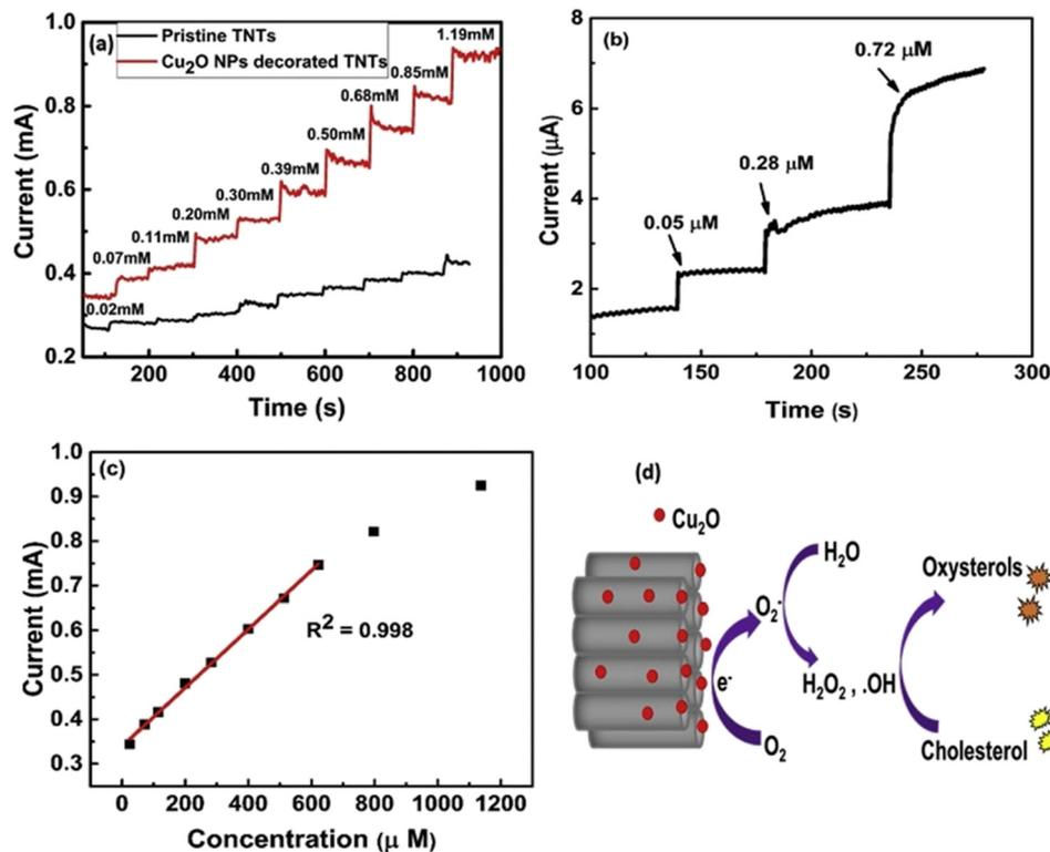
Fig. 7 (a and b) Chronoamperometric plot of the pristine TNTs and Cu<sub>2</sub>O decorated TNTs upon addition of cholesterol; (c) linear calibration curve; (d) diagrammatic presentation of cholesterol oxidation at the electrode surface (reprinted from ref. 92 with permission from Elsevier).
