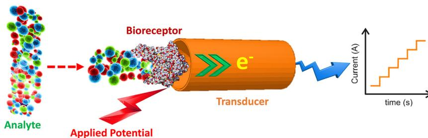
Fig. 3 Visual representation of an amperometric biosensor.
