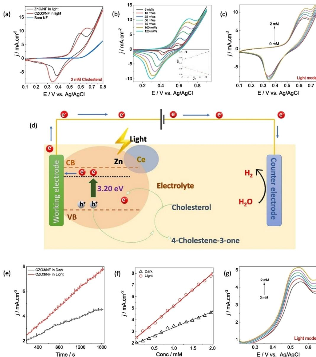
**Fig. 8** The study involving (a–c) CV, (e and f) chronoamperometry, and (g) DPV, along with the proposed (d) mechanism of cholesterol oxidation in photoelectrochemical cholesterol biosensors (reprinted from ref. 113 with permission from Elsevier).
