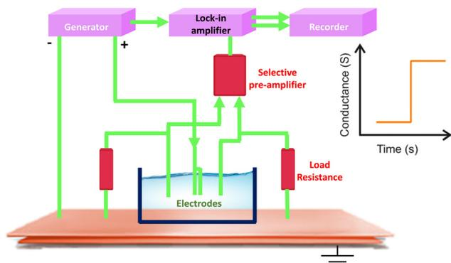
Fig. 4 Schematic representation of a conductometric biosensor.
