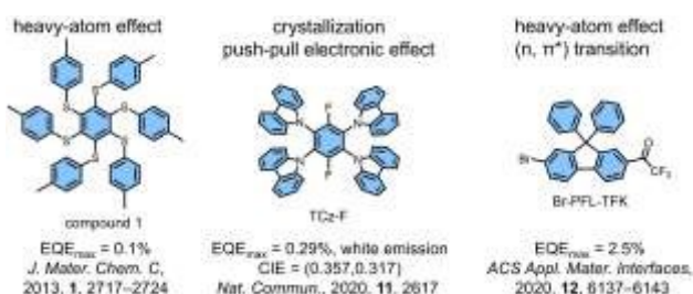
Fig. 5 Molecular structures, mechanisms and corresponding EL performance of the conventional RTP emitters.
