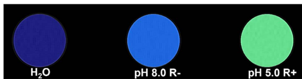
Fig. 9 A coloured T_1 map of the samples taken at 4.7 T and 298 K is in agreement with the observed relaxivities ( T_1 times are 3020 \pm 15 , 2740 \pm 10 , and 2426 \pm 11 ms, respectively). Raw phantom MRI images are available in SI 14.
