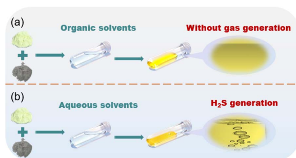
Fig. 9 Illustration of the liquid phase method for preparing SSEs with (a) organic and (b) aqueous solvents.
