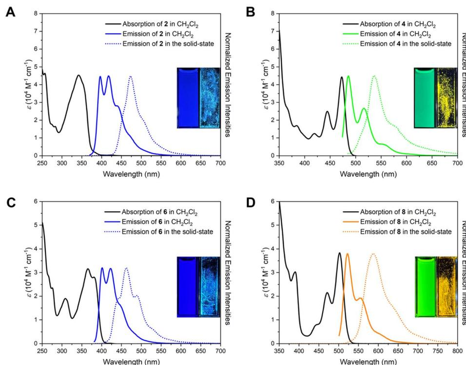
Fig. 5 Solution-state absorption (black lines, 10 mM in CH<sub>2</sub>Cl<sub>2</sub>), solution-state emission (colored solid lines, in CH<sub>2</sub>Cl<sub>2</sub>), and solid-state emission (colored dotted lines) spectra of 2 (A), 4 (B), 6 (C), and 8 (D). The insets show images of each sample in solution- and solid-state under 365 nm irradiation.
