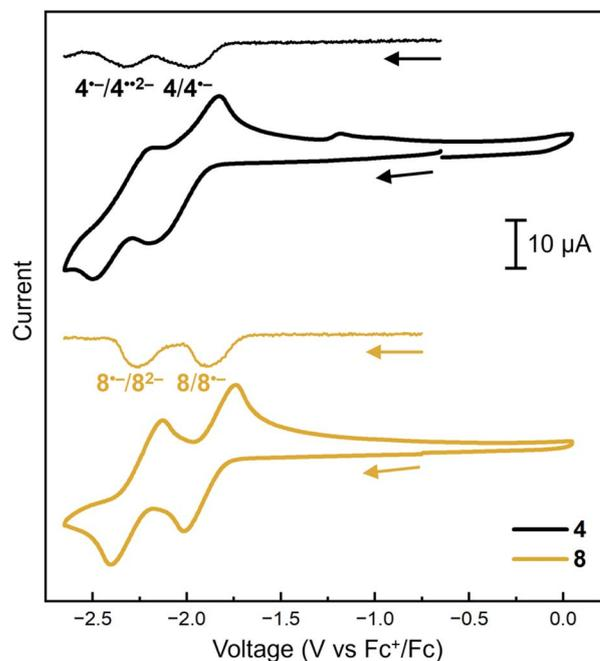
Fig. 7 Cyclic voltammetry and differential pulse voltammetry of 4 (black lines) and 8 (brown lines) in THF with  $n\text{-Bu}_4\text{PF}_6$  (0.2 M) as the supporting electrolyte. Scan rate =  $100 \text{ mV s}^{-1}$ . Sample concentration = 2 mM.
