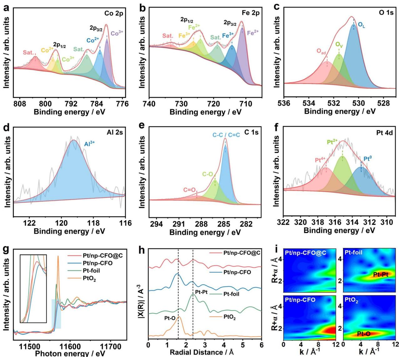
Fig. 3 XPS spectra of the Pt/np-CFO@C electrode: (a) Co 2p, (b) Fe 2p, (c) O 1s, (d) Al 2s, (e) C 1s and (f) Pt 4d. (g) Pt L<sub>3</sub>-edge XANES spectra of Pt/np-CFO@C, Pt/np-CFO, Pt foil and PtO<sub>2</sub>. (h) Pt L<sub>3</sub>-edge EXAFS spectra of Pt/np-CFO@C, Pt/np-CFO, Pt foil and PtO<sub>2</sub>. (i) Pt L<sub>3</sub>-edge WT-EXAFS signals of Pt/np-CFO@C, Pt/np-CFO, Pt foil and PtO<sub>2</sub>.
