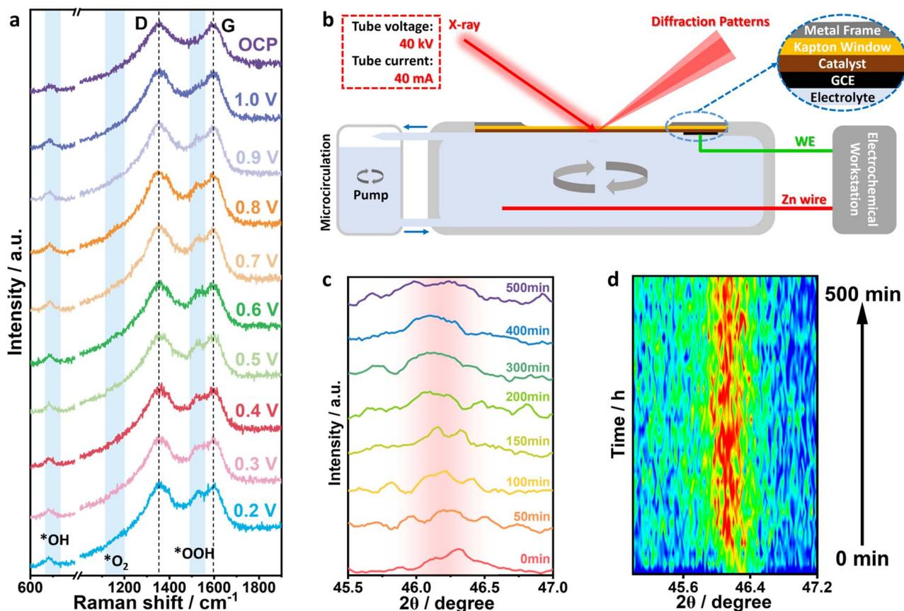
Fig. 7 (a) *In situ* Raman spectra of Pt/np-CFO@C during the ORR. (b) A schematic diagram of an *in situ* X-ray diffractometer applied to a liquid Zn–air battery. (c) Time-resolved *in situ* XRD patterns of a Pt/np-CFO@C-based ZAB during constant current discharge. (d) The corresponding waterfall diagram.
