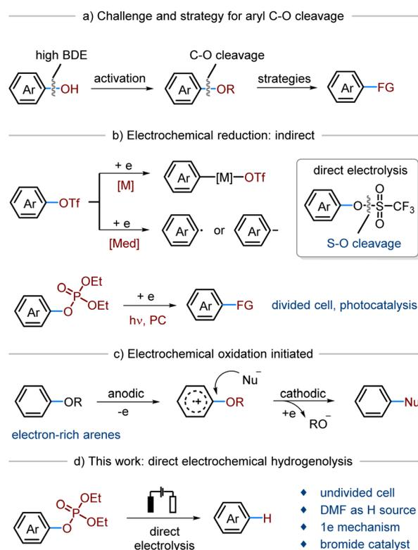
Fig. 1 Introduction of electrochemical aryl C–O cleavage.
