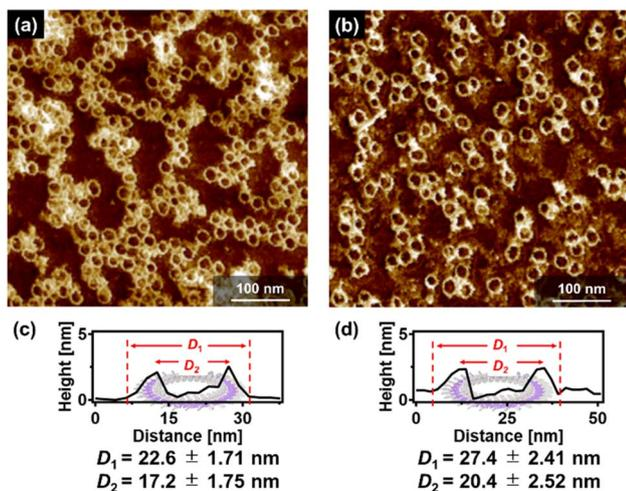
Fig. 5 (a and b) AFM images of  $\text{SP}_{\text{ring}}$  obtained by sonicating a  $\text{SP}_{\text{hel}}$  solution of **1** ( $c = 50 \mu\text{M}$ ) in (a) MCH and (b) MCH including 0.7% (v/v) THF. (c and d) AFM cross-sectional analyses of representative  $\text{SP}_{\text{ring}}$  structures in (a) and (b), respectively. Average outer diameters ( $D_1$ ) and top-to-top diameters ( $D_2$ ) were determined from 100  $\text{SP}_{\text{ring}}$  structures.
