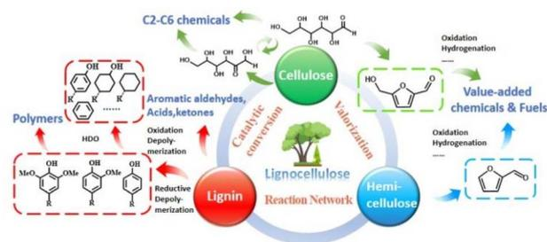
Fig. 1 Catalytic conversion network for value-added utilization of lignocellulosic biomass. Reproduced with permission.<sup>5</sup> Copyright 2023, the Royal Society of Chemistry.
