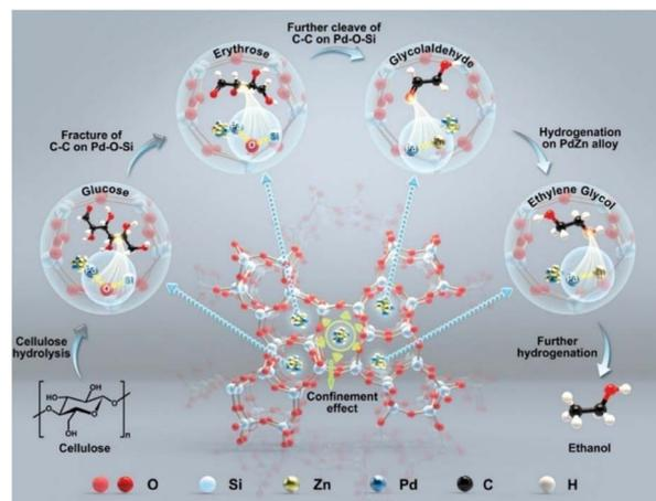
Fig. 9 Presumptive reaction mechanism for the cellulose hydrogenolysis to ethanol over PdZn<sub>0.5</sub>@S-1 catalyst. Reproduced with permission.<sup>190</sup> Copyright 2025, Wiley-VCH.
