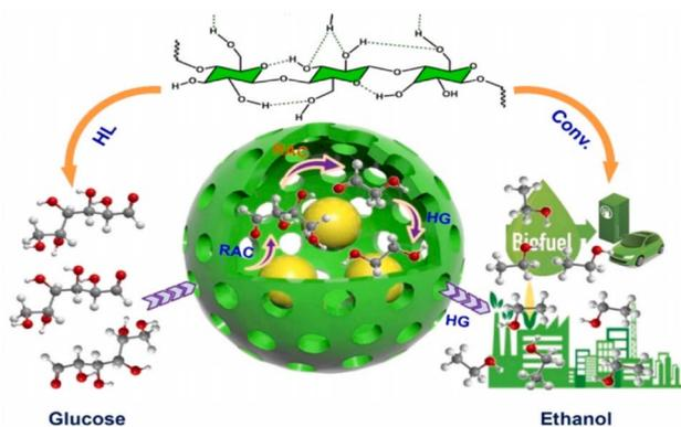
Fig. 8 Schematic representation of cascade steps and active site locations of cellulose hydrogenation to ethanol over Pd@Al<sub>3</sub>-SiO<sub>2</sub> catalyst. Reproduced with permission.<sup>189</sup> Copyright 2025, Elsevier.
