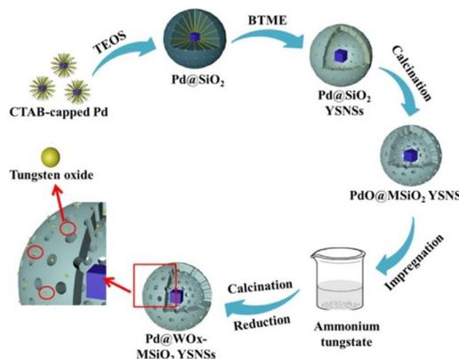
Fig. 6 Schematic representation of the synthesis of Pd@WO<sub>x</sub>-MSiO<sub>2</sub> YSNSs. Reproduced with permission.<sup>191</sup> Copyright 2021, American Chemical Society.
