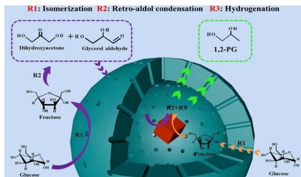
Fig. 7 The possible reaction route of glucose hydrogenolysis on Pd@Al-MSiO<sub>2</sub> YSNSs. Reproduced with permission.<sup>192</sup> Copyright 2020, Elsevier.
