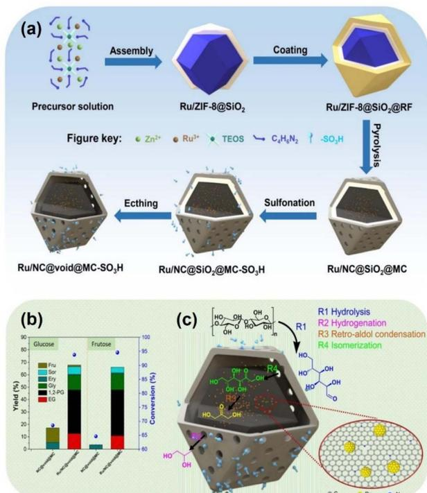
Fig. 5 (a) Preparation process of Ru/NC@void@MC-SO<sub>3</sub>H catalyst; (b) performance evaluation of glucose and fructose on NC@void@MC and Ru/NC@void@MC; (c) possible reaction mechanism of cellulose generating 1,2-PG on Ru/NC@void@MC-SO<sub>3</sub>H. Reproduced with permission.<sup>127</sup> Copyright 2023, Elsevier.
