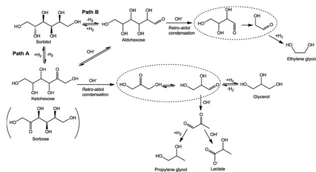
Fig. 4 The proposed reaction pathway for the hydrogenolysis of sorbitol to produce  $\text{C}_2$  and  $\text{C}_3$  products in the presence of alkaline and metal catalysts. Reproduced with permission.<sup>173</sup> Copyright 2016, the Royal Society of Chemistry.
