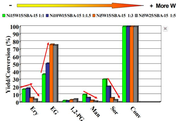
Fig. 3 The variation of product distribution on the Ni–W/SBA-15 bimetallic catalyst with the Ni/W mass ratio. Conv, Ery, EG, 1,2-PG, Mann, and Sor represent the cellulose conversion rate and the yields of erythritol, ethylene glycol, 1,2-propanediol, mannitol, and sorbitol, respectively. Reproduced with permission.<sup>45</sup> Copyright 2014, Elsevier.
