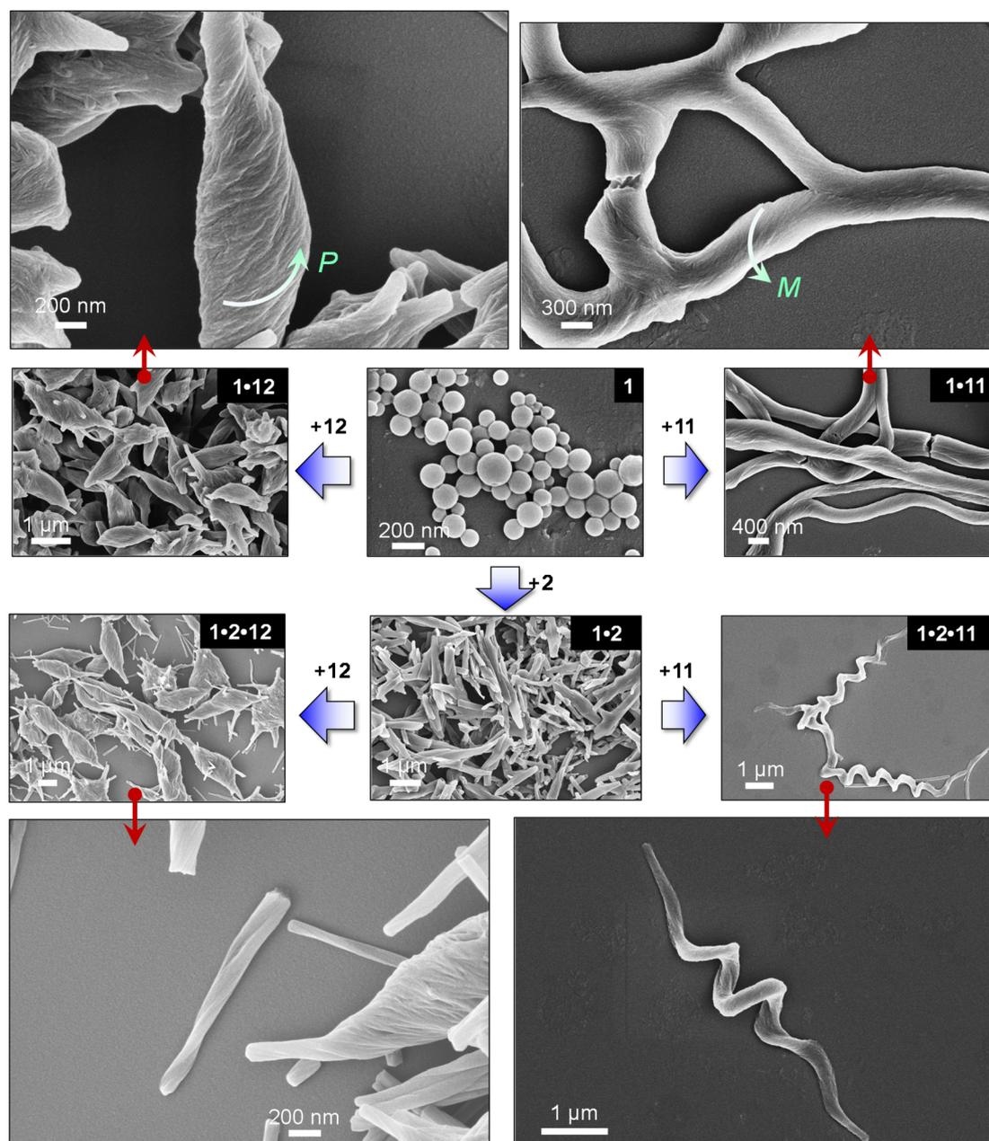
Fig. 6 SEM images of **1** ( $f_w = 80$  vol%), **1**·**2** ( $f_w = 80$  vol%, 1 : 1), **1**·**11** ( $f_w = 80$  vol%, 1 : 1), **1**·**12** ( $f_w = 80$  vol%, 1 : 1), **1**·**2**·**11** ( $f_w = 80$  vol%, 1 : 1 : 1), and **1**·**2**·**12** ( $f_w = 80$  vol%, 1 : 1 : 1) respectively. [**1**] = 0.1 mM.
