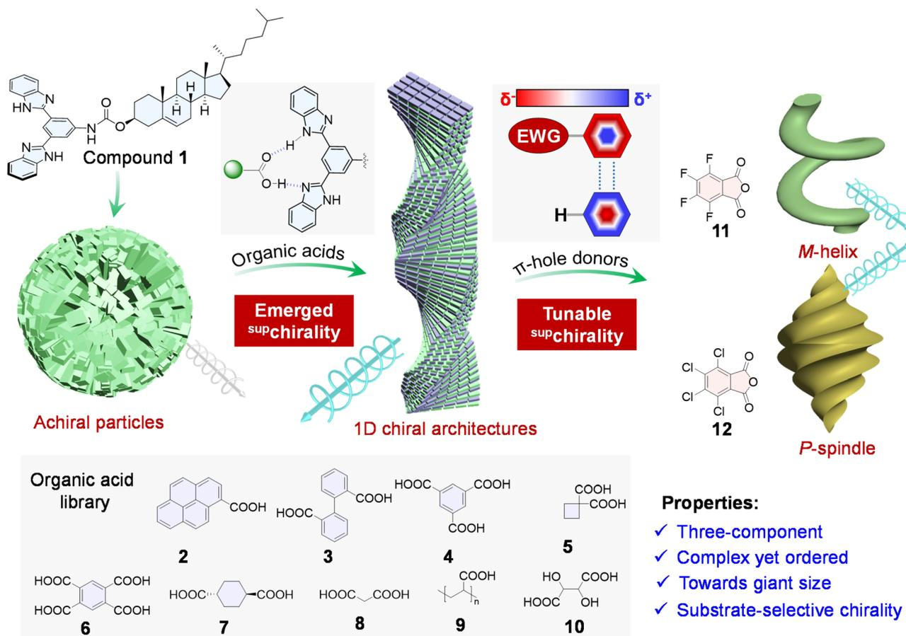
Scheme 1 Molecular structures of compound 1, achiral acids (2–10), and  $\pi$ -hole donors (11, 12), accompanied by the evolution of chiroptical properties and supramolecular architectures throughout the coassembly process.
