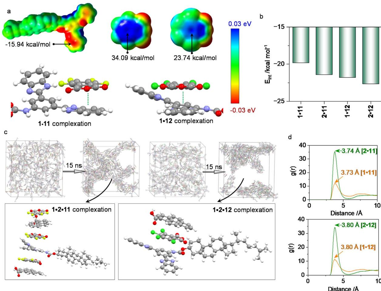
Fig. 5 (a) Electrostatic potential maps of **1**, **11**, and **12**, as well as the DFT-optimized structures of the **1·11** and **1·12** complexes. (b) The interaction energies for the formation of the **1·11**, **2·11**, **1·12**, and **2·12** complexes. (c) MD results. Aggregation behaviors within the simulation boxes at 0 ns and 15 ns for comparison. (d) RDF profiles of distances for the intermolecular interaction between **1·11**, **2·11**, **1·12** and **2·12**.
