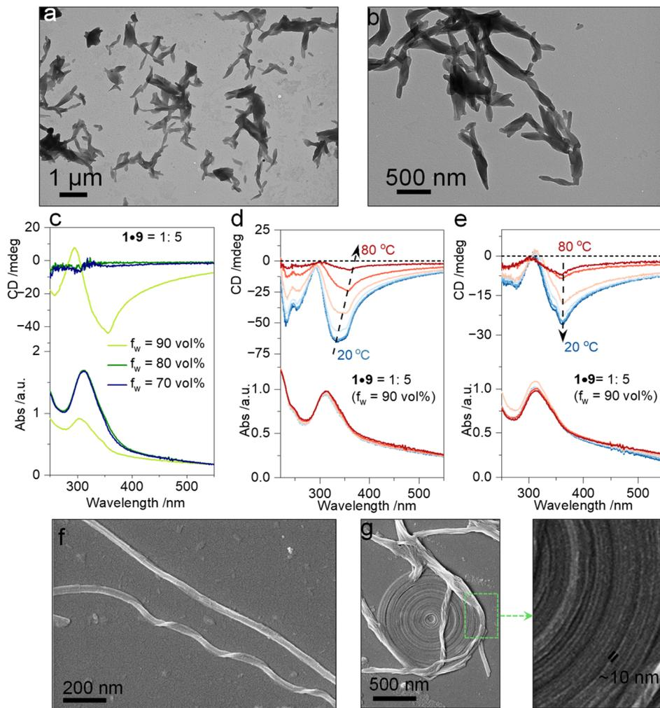
Fig. 3 (a and b) TEM images of 1·9 coassemblies ( $c = 1$  mM, ratio = 1 : 5, based on the monomer,  $f_w = 90$  vol%). (c) CD spectra of 1·9 coassemblies (1 : 5, based on the monomer). (d and e) Heating and cooling CD curves of 1·9 coassemblies. (f and g) SEM image of 1·TA ( $f_w = 70$  vol%, 1 : 5 by molar ratio) coassemblies.  $[1] = 1$  mM.
