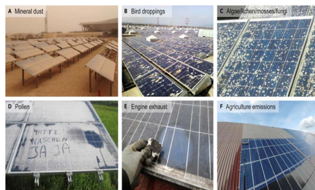
Fig. 15 (a–f) Overview of different soiling types with exemplary photographs of the soiling of the PV panels. Reproduced from ref. 83–86 with permission.
