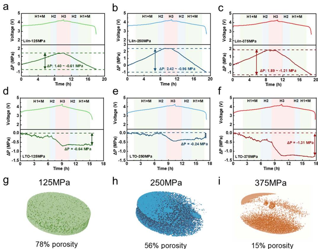
Fig. 2 Pressure changes during charging and discharging. *In situ* pressure measurement curves and voltage profiles of the (a) LiIn-125 MPa, (b) LiIn-250 MPa, (c) LiIn-375 MPa, (d) LTO-125 MPa, (e) LTO-250 MPa, and (f) LTO-375 MPa during the first charging and discharging. (g–i) Three-dimensional nano-CT volume rendering images of the composite cathode under different stacking pressures. The colored regions represent pores.
