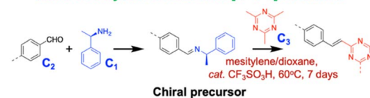
Scheme 1 (a) Previously reported chirality-induced transamination via a reversible aldimine condensation reaction. (b) Currently used chirality-induced imine-to-vinylene conversion via an irreversible aldol condensation reaction. Reaction conditions: 60 °C, 7 days, CF_3SO_3H (catalyst), mesitylene/dioxane (1/1, v/v).
