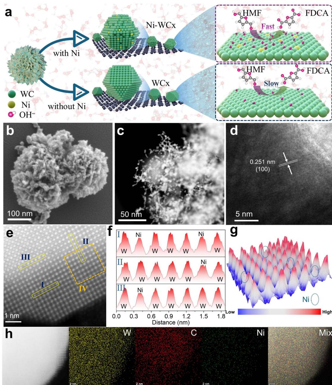
**Fig. 1** Morphological and structural characterization of the synthesized materials. (a) Schematic illustration of Ni-WCx and WCx, highlighting the atomic engineering effect toward HMFOR. (b) SEM, (c) TEM, and (d) HRTEM images of Ni-WCx. (e) HAADF-STEM image of Ni-WCx, revealing atomic-scale features. (f) Corresponding intensity profile and (g) 3D atomic-resolution topographic representation derived from IV region in (e). (h) Elemental mapping of W, C and Ni in Ni-WCx.
