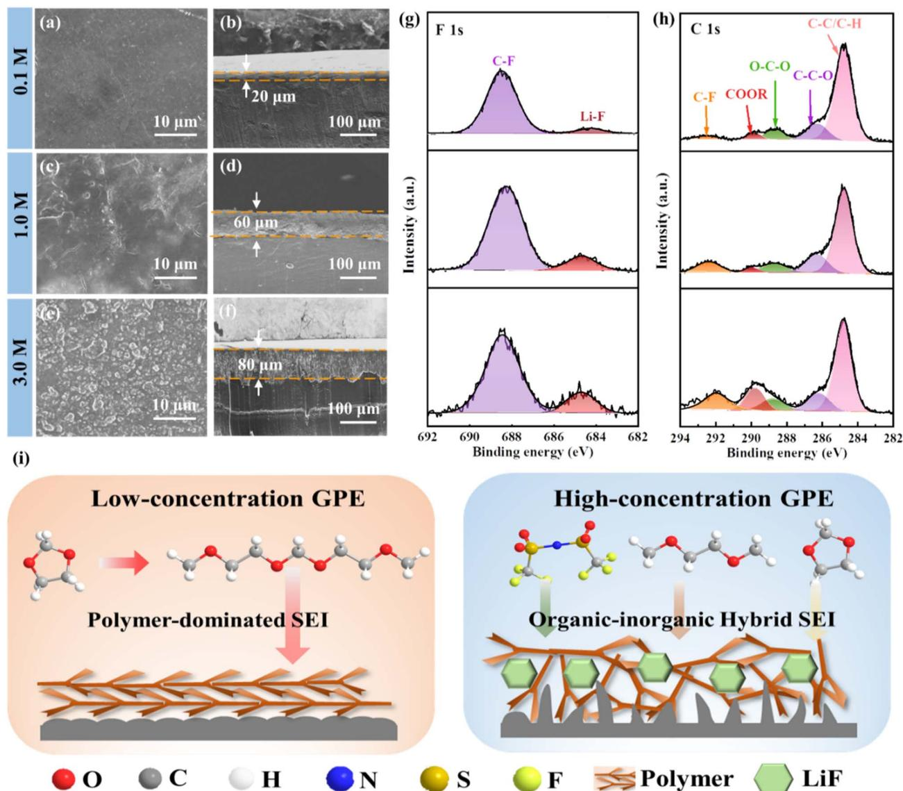
Fig. 3 Impacts of electrolyte concentrations on Li anodes in TAQB-Li batteries after 200 cycles. SEM images of the (a, c and e) surface and (b, d and f) cross-section and XPS spectra of (g) F 1s and (h) C 1s of the cycled Li anodes using different concentration GPEs. (i) Schematic diagrams of the SEI formation and decomposition of low- and high-concentration GPEs.
