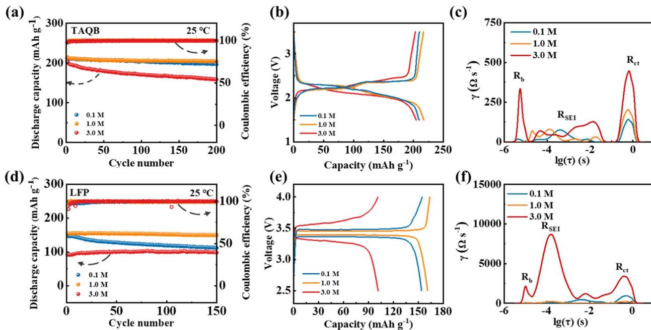
Fig. 2 Electrochemical performance comparison of TAQB-Li and LFP-Li batteries utilizing GPEs with varying LiTFSI concentrations of 0.1, 1.0, and 3.0 M at 0.5C and 25 °C. (a and d) Cycling performance, (b and e) charge–discharge profiles, (c and f) corresponding DRT plots derived from EIS data collected over the frequency range of  $10^6$  to 1 Hz for (a–c) TAQB-Li and (d–f) LFP-Li batteries.
