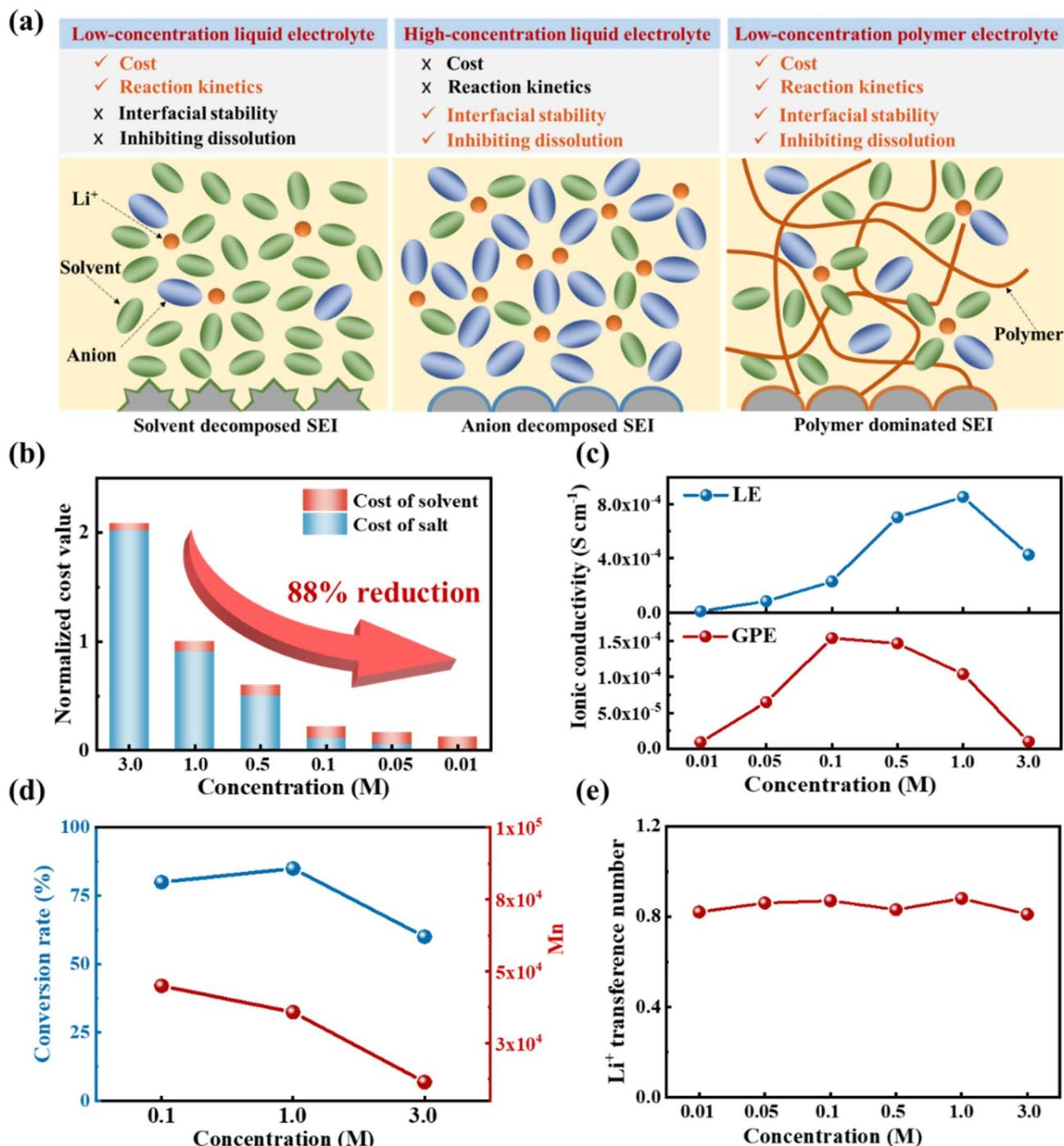
Fig. 1 (a) Schematic representations of various electrolyte systems. (b) Estimated electrolyte cost comparison for LEs with different salt concentrations. (c) Ionic conductivities comparison between LEs and GPEs. (d) Conversion rate of DOL to poly-DOL (PDOL) and the number-average molecular weight ( $M_n$ ) of PDOL in GPEs. (e) Li-ion transference numbers of GPEs with different LiTFSI concentrations ranging from 0.01 M to 3.0 M.
