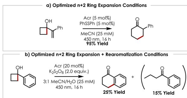
Scheme 4 Optimized conditions for (a) *n*+2 ring expansion and (b) *n*+2 ring expansion + rearomatization. <sup>a</sup>Yields determined by <sup>1</sup>H NMR spectroscopy. Full optimization tables are available in the SI (Tables S5 and S8).
