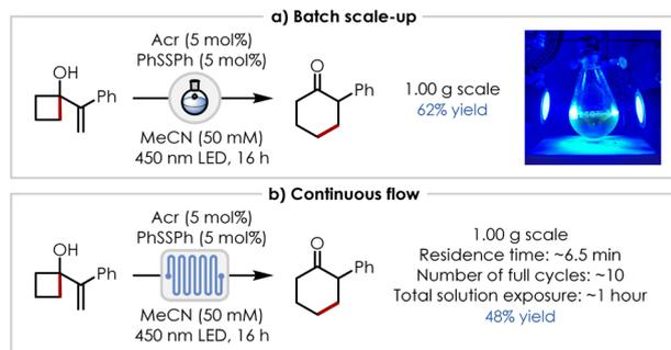
Scheme 5 Scale-up of  $n+2$  ring expansion: (a) batch scale up, (b) continuous flow. <sup>a</sup>Details of setup, additional parameters, and equations for their calculation are given in the SI.
