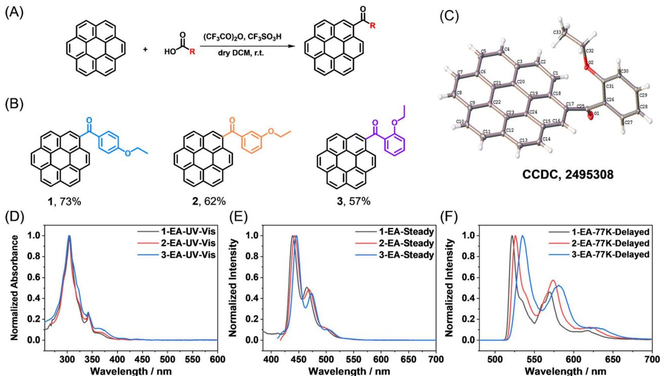
Fig. 2 (A) Synthesis of coronene derivatives *via* acid-catalyzed Friedel–Crafts reaction. (B) Chemical structure of compounds 1, 2, and 3, as well as the isolation yields. (C) Single crystal structure of compound 3. (D) UV-Vis absorption spectra of 1, 2, 3 in ethyl acetate (EA) solution. (E) Steady-state spectra of compounds 1, 2, 3 in EA solution at room temperature. (F) Delayed emission (1 ms delay) spectra of 1, 2, 3 in EA solution at 77 K.
