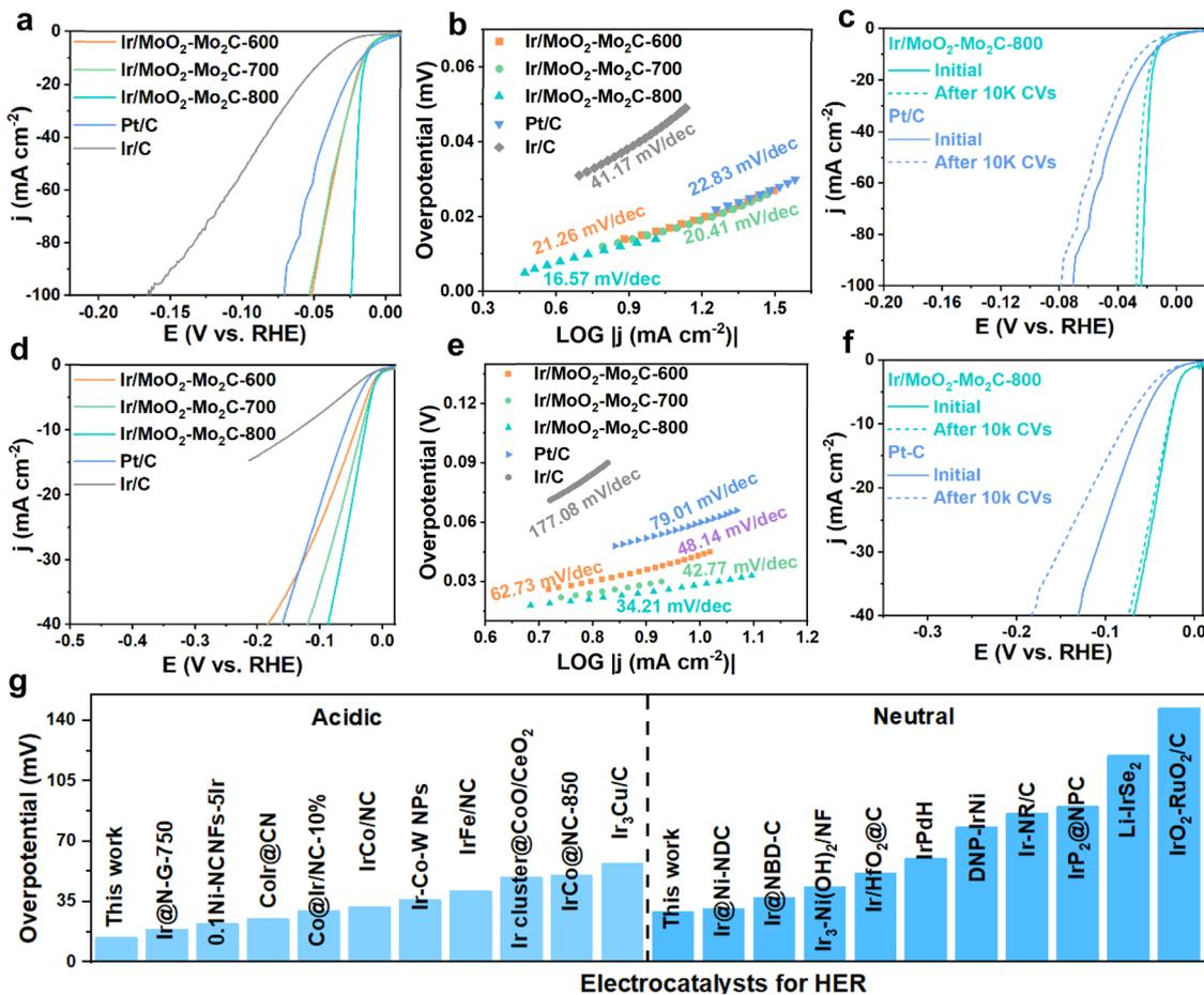
Fig. 5 (a and b) HER polarization curves and (c and d) Tafel plots of the as-synthesized samples in 0.5 M H<sub>2</sub>SO<sub>4</sub> and in 1.0 M PBS. (e and f) Polarization curves for Ir/MoO<sub>2</sub>-Mo<sub>2</sub>C-800 before and after CV potential cycles in 0.5 M H<sub>2</sub>SO<sub>4</sub> and in 1.0 M PBS. (g) Performance comparison between the Ir/MoO<sub>2</sub>-Mo<sub>2</sub>C-800 and reported advanced HER catalysts in all-pH hydrogen evolution.
