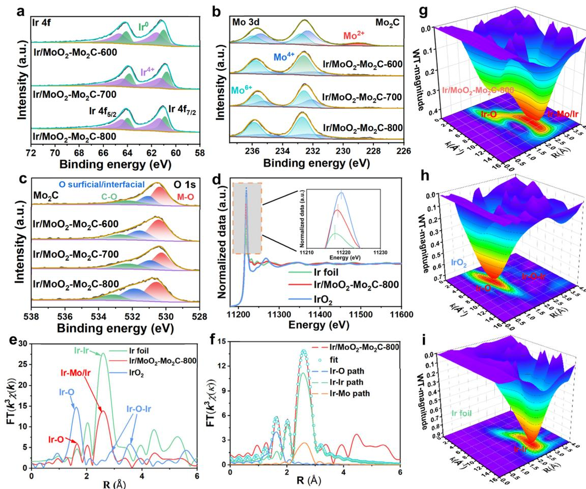
Fig. 3 XPS spectra of (a) Ir 4f, (b) Mo 3d, and (c) O 1s for Ir/MoO<sub>2</sub>-Mo<sub>2</sub>C-600, Ir/MoO<sub>2</sub>-Mo<sub>2</sub>C-700, Ir/MoO<sub>2</sub>-Mo<sub>2</sub>C-800, and Mo<sub>2</sub>C. (d) Ir L<sub>3</sub>-edge XANES spectra and (e and f) corresponding FT-EXAFS curves of Ir/MoO<sub>2</sub>-Mo<sub>2</sub>C-800, Ir foil, and IrO<sub>2</sub>. EXAFS wavelet transform plots of (g) Ir/MoO<sub>2</sub>-Mo<sub>2</sub>C-800, (h) IrO<sub>2</sub>, and (i) Ir foil.
