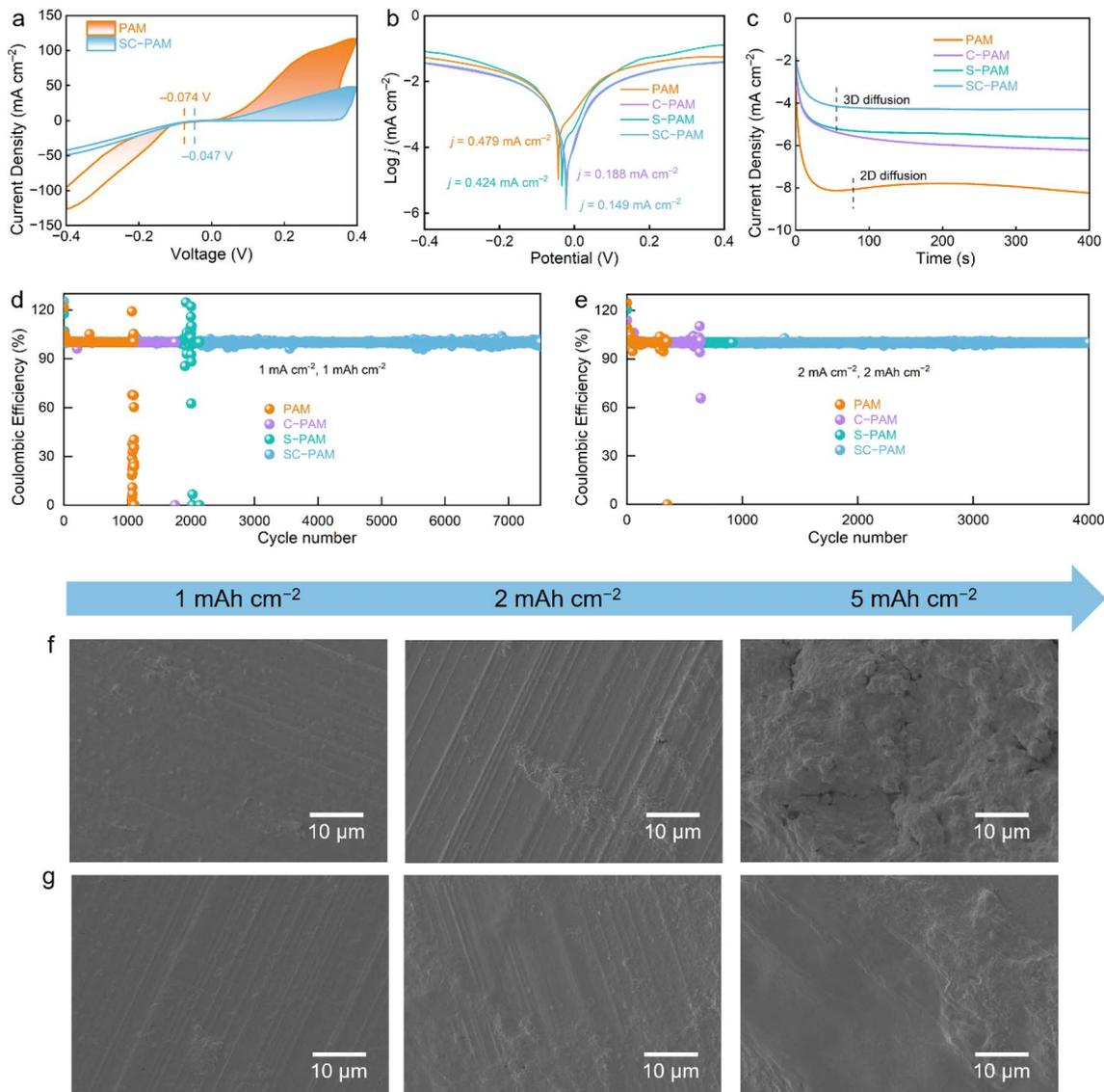
Fig. 4 (a) Cyclic voltammograms of Zn||Cu cells using PAM and SC-PAM hydrogel electrolytes at  $1 \text{ mV s}^{-1}$ . (b) Tafel plots. (c) CA test of Zn||Cu cells at a constant voltage of  $-150 \text{ mV}$ . (d and e) Long-term performance of Zn||Cu cells. SEM images of plating Zn on a Cu current collector with different areal capacities in (f) PAM and (g) SC-PAM.
