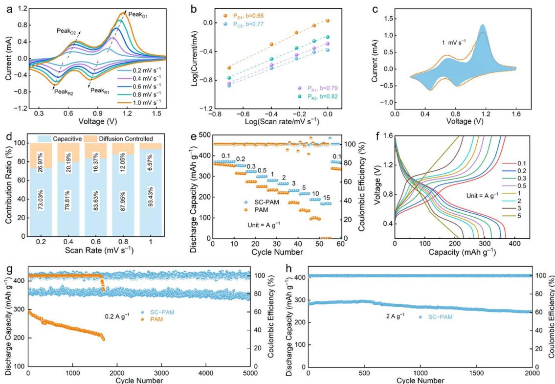
Fig. 6 Charge storage kinetics of the Zn||SC-PAM||V<sub>2</sub>O<sub>5</sub> cell. (a) CV curves. (b) Calculated *b* values. (c) Capacitive contribution at 1 mV s<sup>-1</sup>. (d) Ratios of capacitive and diffusion-controlled contribution at various scan rates. (e) Rate performance. (f) GCD curves. Long-term cycling performance at (g) 0.2 A g<sup>-1</sup> and (h) 2 A g<sup>-1</sup>.
