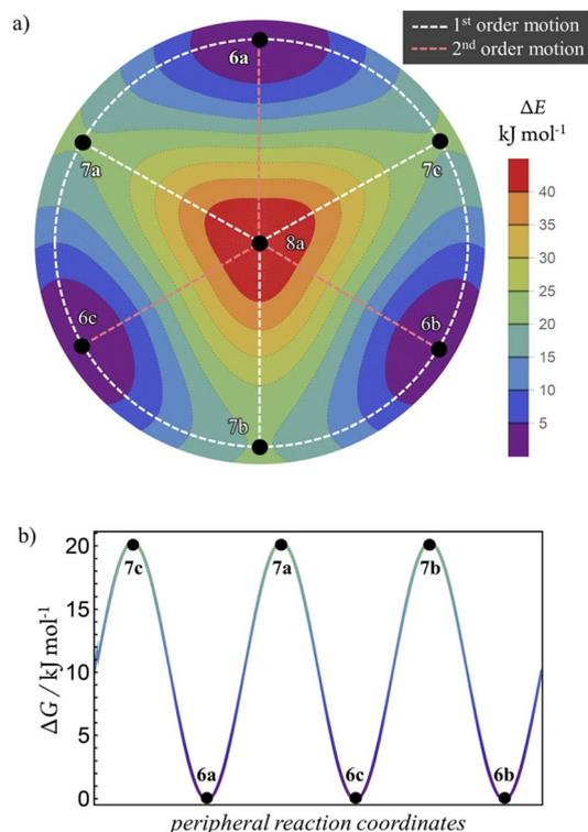
Fig. 10 Minimal interpolated approximation of the PES for tautomerism in free-base subporphyrin monoanion using the  $S_3B_1$  partitioning approach. (a) The 2D PES overlain by the reaction graph (labelled points and dashed lines). (b) The 1D periodic PES interpolated from genera 6 and 7 – the outer periphery in (a) with the same energy scale.
