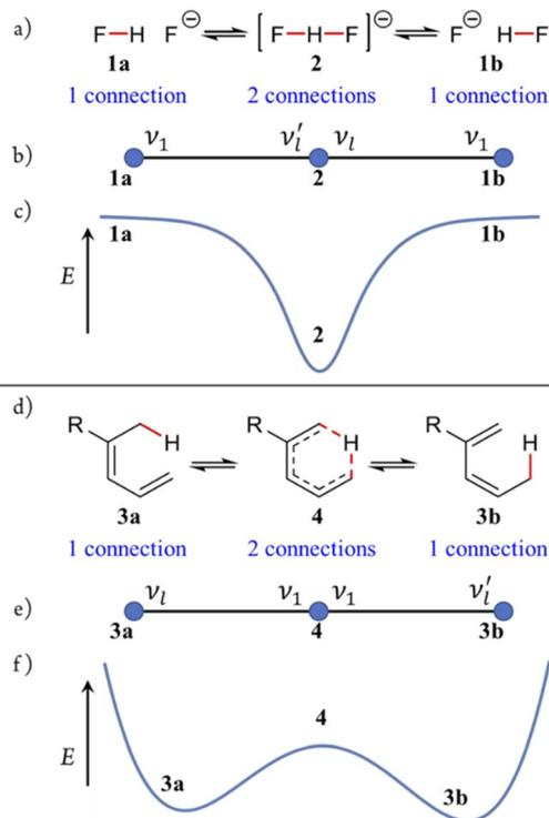
Fig. 4 Two desmotropic chemical reactions, reaction-graph representations, and potential energy surface relationships for (a–c) dissociation ( $R_{de}^2$  process) of bifluoride anion 2 into [HF + fluoride] 1, and (d–f) the [1,5] sigmatropic rearrangement ( $R_{de}^1$  process) of 3a to 3b via 4. Coloured atom connections are permuting.  $\nu_l$  denotes local bond-stretching modes.  $\nu_1$  denotes the imaginary mode.
