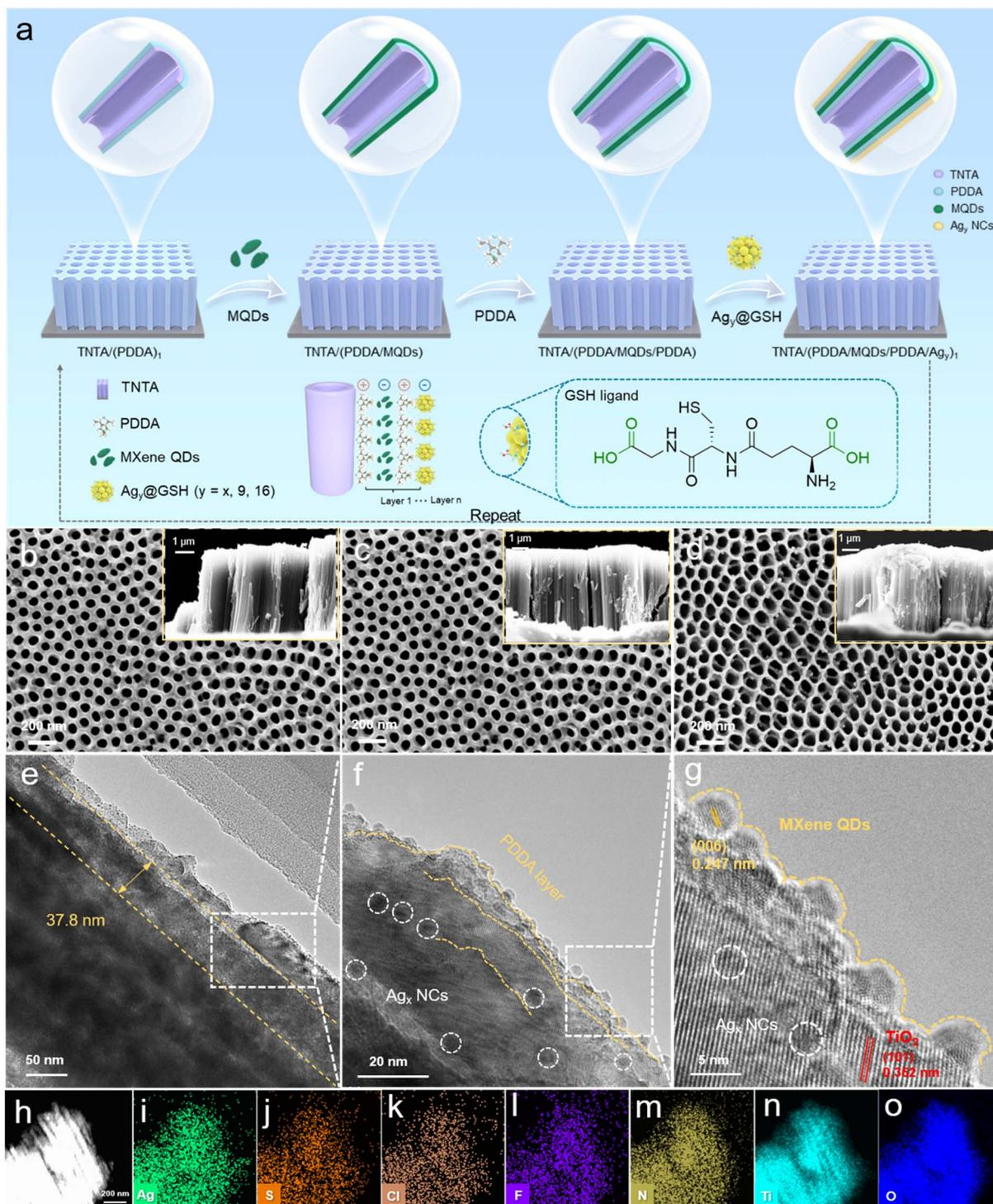
Fig. 1 (a) Schematic demonstration of LbL assembly of TNTA/(P/MQDs/P/Ag<sub>x</sub>)<sub>n</sub> (y = x, 9, 16) multilayer heterostructures. SEM images of (b) TNTA, (c) TNTA/(Ag<sub>x</sub>)<sub>6</sub> and (d) TNTA/(P/MQDs/P/Ag<sub>x</sub>)<sub>6</sub> with corresponding cross-sectional images. (e) TEM and (f & g) HRTEM images of TNTA/(P/MQDs/P/Ag<sub>x</sub>)<sub>6</sub> with (h–o) corresponding mapping results.
