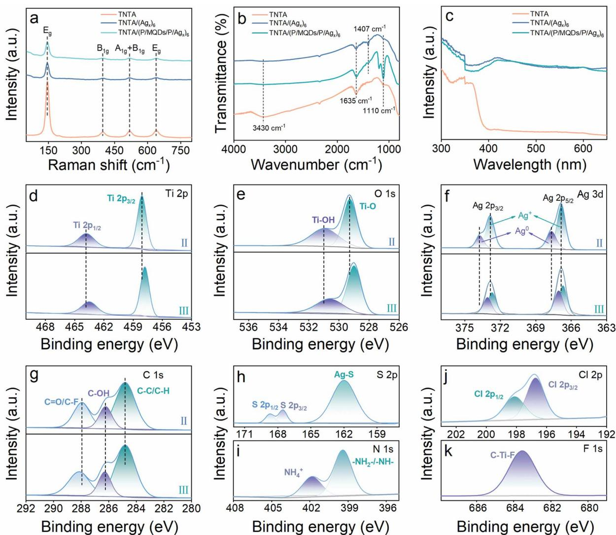
Fig. 2 (a) Raman, (b) FTIR and (c) DRS results of TNTA, TNTA/(Ag<sub>x</sub>)<sub>6</sub> and TNTA/(P/MQDs/P/Ag<sub>x</sub>)<sub>6</sub>; high-resolution (d) Ti 2p, (e) O 1s, (f) Ag 3d, (g) C 1s of (II) TNTA/(Ag<sub>x</sub>)<sub>6</sub> and (III) TNTA/(P/MQDs/P/Ag<sub>x</sub>)<sub>6</sub>, and high-resolution (h) S 2p, (i) N 1s, (j) Cl 2p and (k) F 1s of TNTA/(P/MQDs/P/Ag<sub>x</sub>)<sub>6</sub>.
