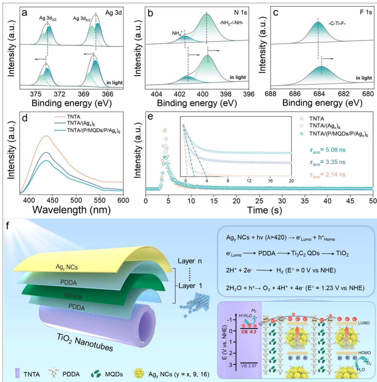
Fig. 5 High-resolution *in situ* XPS spectra of (a) Ag 3d, (b) N 1s and (c) F 1s for TNTA/(P/MQDs/P/Ag<sub>x</sub>)<sub>6</sub>; (d) PL and (e) TRPL results of TNTA, TNTA/(Ag<sub>x</sub>)<sub>6</sub> and TNTA/(P/MQDs/P/Ag<sub>x</sub>)<sub>6</sub>; (f) schematic illustration of the PEC water oxidation mechanism of TNTA/(P/MQDs/P/Ag<sub>x</sub>)<sub>n</sub> photoanodes.
