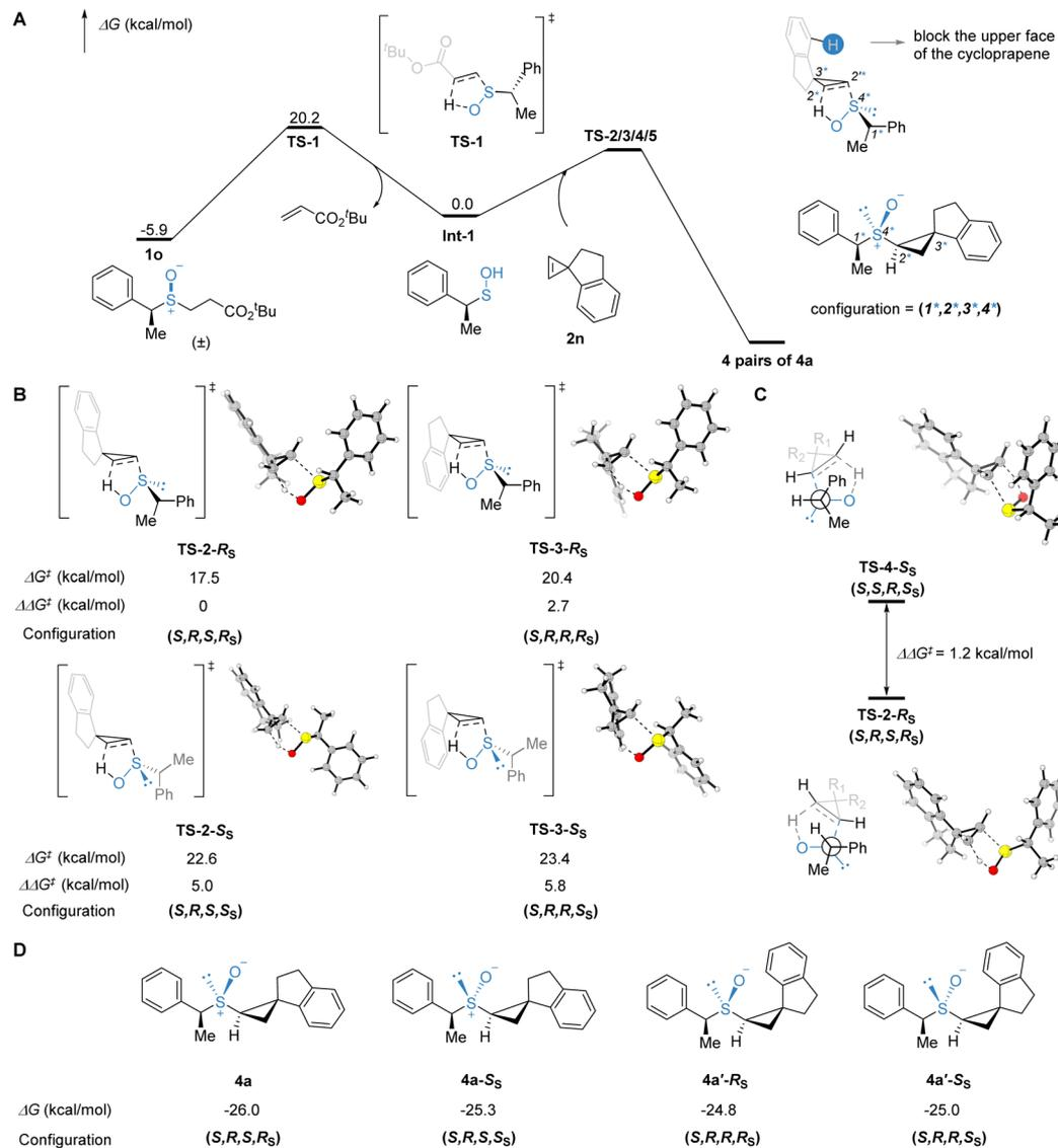
Fig. 3 Computational studies. DFT calculated reaction pathways at M062X/def2-TZVP/SMD(Toluene)//B3LYP-D3/def2-SVP level. All energies are in kcal mol<sup>-1</sup>. (A): Overall energy profile. (B): Transition states regarding *endo/exo* and facial selectivity. (C): Side selectivity of carbon 2\* vs. 2'.
