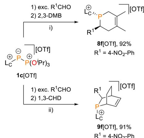
Scheme 4 Phospha-Diels-Alder type trapping reactions of *in situ* prepared imidazolium-substituted phosphalkene  $2f[OTf]$  with 2,3-dimethylbuta-1,3-diene (2,3-DMB) and 1,3-cyclohexadiene (1,3-CHD); reagents and conditions: (i) – OP(O<sup>i</sup>Pr)<sub>3</sub>, CH<sub>2</sub>Cl<sub>2</sub>, r.t., 16 h, 92%; (ii) – OP(O<sup>i</sup>Pr)<sub>3</sub>, CH<sub>2</sub>Cl<sub>2</sub>, r.t., 16 h, 91%.
