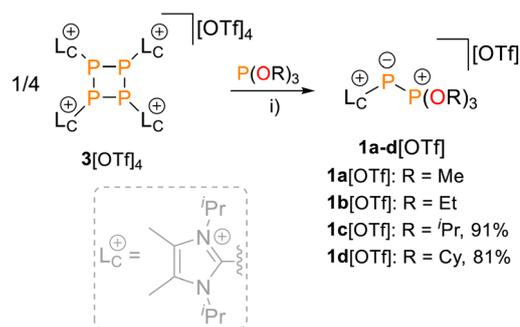
Scheme 1 Nucleophilic fragmentation of **3** $[\text{OTf}]_4$  with organophosphites  $\text{P(OR)}_3$  (**R** = Me, Et, <sup>*i*</sup>Pr, Cy); reagents and conditions: (i) +4.2  $\text{P(OR)}_3$ ,  $\text{CH}_3\text{CN}$  or  $\text{CD}_2\text{Cl}_2$ , r.t., 16 h, 91% (**1c** $[\text{OTf}]$ , **R** = <sup>*i*</sup>Pr), 16 h, 81% (**1d** $[\text{OTf}]$ , **R** = Cy).
