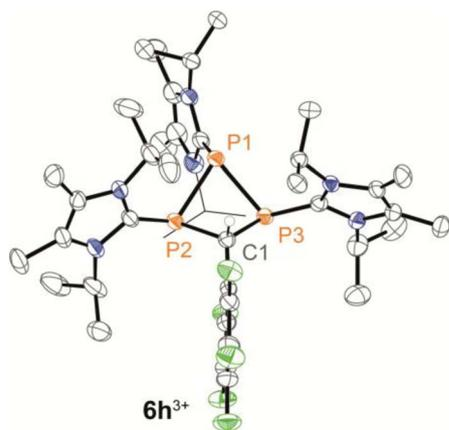
Fig. 4 Molecular structures of **6h**<sup>3+</sup> in **6h**[OTf]<sub>3</sub>·C<sub>6</sub>H<sub>5</sub>F; selected hydrogen atoms and anions are omitted for clarity, and thermal ellipsoids are displayed at 50% probability (100 K), one <sup>1</sup>Pr of the L<sub>C</sub> group at P1 is shown in wireframe for clarity; selected bond lengths (Å) and angles (°): for **6h**<sup>3+</sup>: P1–P2 2.2354(8), P1–P3 2.2540(9), P2–C1 1.890(2), P3–C1 1.904(3), P2–P1–P3 73.56(3), P2–C1–P3 90.24(10).
