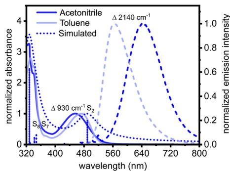
Fig. 2 Electronic absorption (solid lines) and emission (dashed lines;  $\lambda_{\text{exc}} = 450 \text{ nm}$ ) spectra of  $2^t\text{BuCzDPPZ}$  in acetonitrile (blue) and toluene (light blue) together with its simulated absorption spectra (dotted lines, blue).
