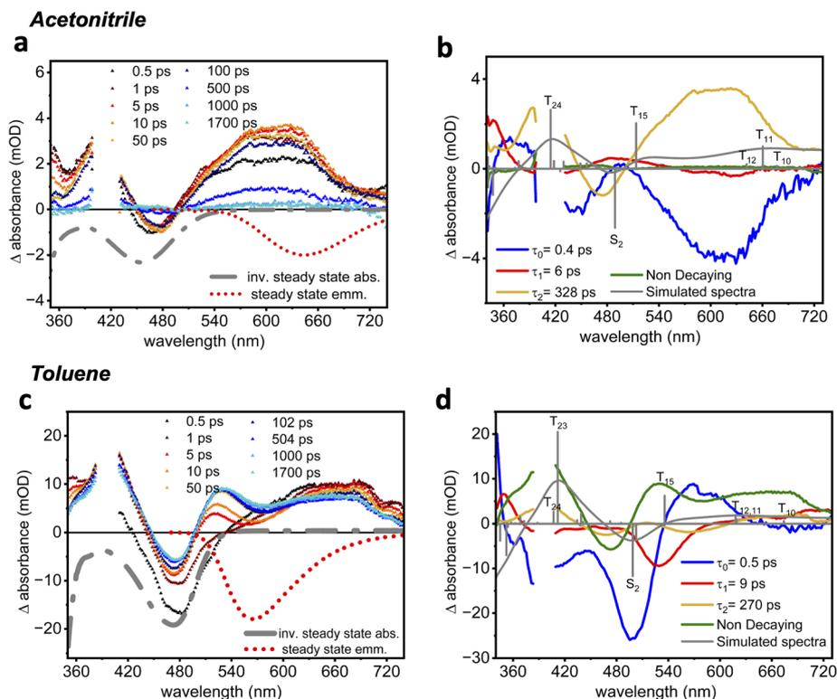
Fig. 4 (a and c) Transient absorption spectra of  $2^t\text{BuCzDPPZ}$  in acetonitrile (a) and toluene (c) following excitation at 400 nm. (b and d) Decay-associated spectra (DAS) in the wavelength range of 350 to 740 nm with its simulated TD (DFT) calculated spectra in acetonitrile (b) and toluene (d).
