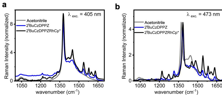
Fig. 3 Resonance Raman spectra of  $2^t\text{BuCzDPPZ}$  and  $2^t\text{BuCzDPPZRhCp}^*$  in acetonitrile excited at (a) 405 nm and (b) 473 nm. All spectra are recorded in solution, normalized to the solvent band (acetonitrile) at  $1370\text{ cm}^{-1}$  and with respect to the absorption coefficient of the corresponding excitation wavelength.
