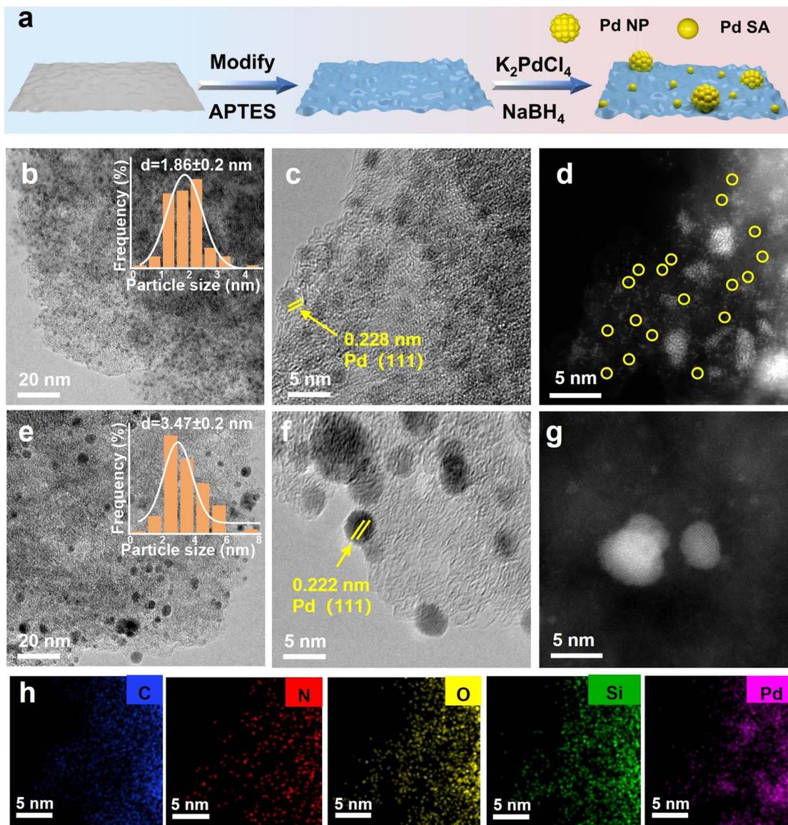
Fig. 1 Characterization of Pd/C-NH<sub>2</sub> and Pd/C. (a) Schematic illustration for the synthetic processes of Pd/C-NH<sub>2</sub>. (b, c, e and f) TEM and HRTEM images of Pd/C-NH<sub>2</sub> and Pd/C. (d and g) AC-STEM images of Pd/C-NH<sub>2</sub> and Pd/C. (h) EDS elemental distribution diagram of Pd/C-NH<sub>2</sub>.
