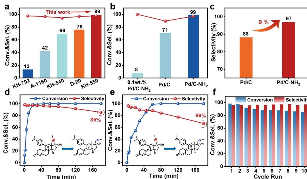
Fig. 4 Catalytic activity evaluation. (a) Comparison of catalytic performance of catalysts modified with different silane coupling agents. (b) Comparison of conversion of Pd/C-NH<sub>2</sub>, Pd/C and 0.1 wt% Pd/C-NH<sub>2</sub>. (c) Comparison of selectivity between Pd/C-NH<sub>2</sub> and Pd/C. (d and e) Time curves of Pd/C-NH<sub>2</sub> and Pd/C. (f) Stability cyclic test of Pd/C-NH<sub>2</sub>. Reaction conditions: 250 mg mifepristone, 6 mg catalyst, 25 °C, 0.1 MPa.
