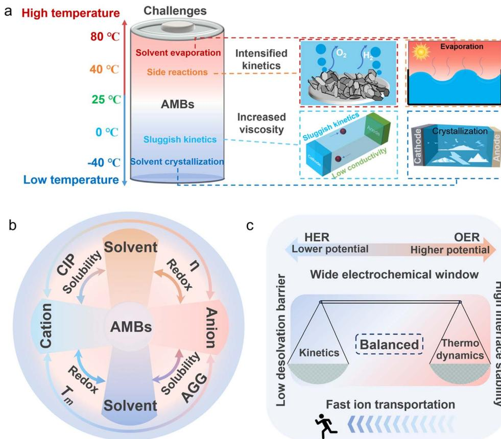
Fig. 2 (a) High- and low-temperature challenges faced by AMBs. (b) An electrolyte–component interaction map ( $T_m$ : melting point;  $\eta$ : viscosity; CIP: contact ion pair; AGG: aggregates). (c) Kinetic and thermodynamic equilibrium.
