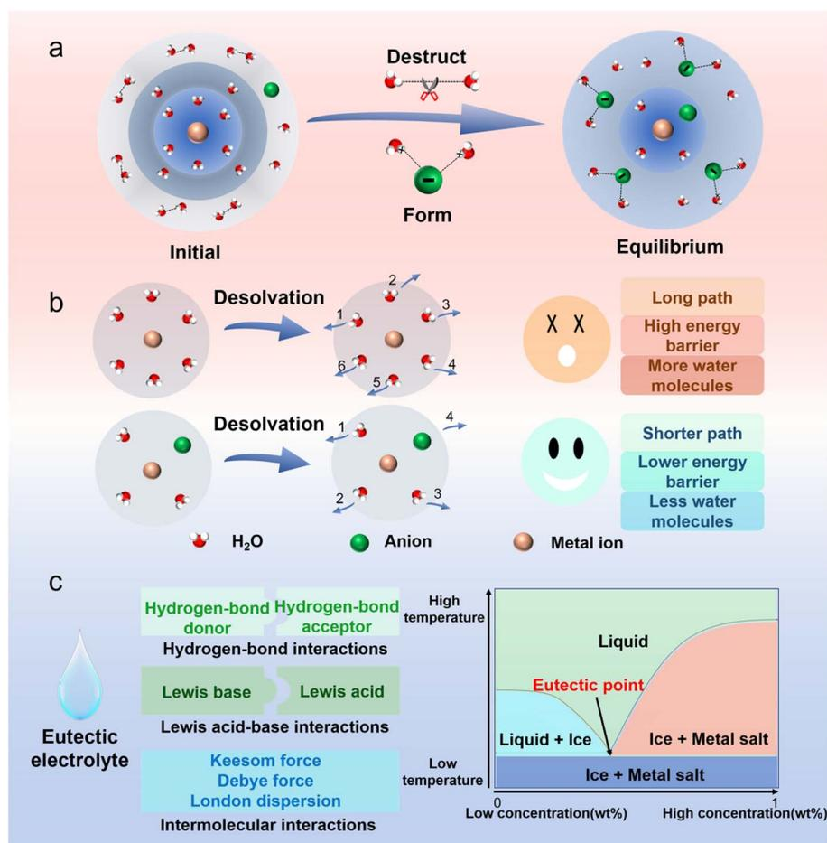
Fig. 4 (a) Ion coordination in electrolytes. (b) Desolvation under different conditions. (c) The principle of eutectic electrolytes.
