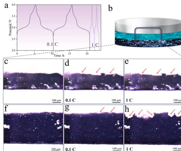
Fig. 6 *Operando* microscopic observation of quasi-solid-state and liquid-state SIBs during operation. (a) Charge and discharge curves of SIBs at different current densities. (b) Schematic illustration of the observation view. Images of the quasi-solid-state SIBs in the (c) initial and (d) charged state at a current density of 0.1C and the (e) charged state at 1C. Image of the liquid-state SIBs in the (f) initial and (g) charged state at a current density of 0.1C and (h) charged state at 1C.
