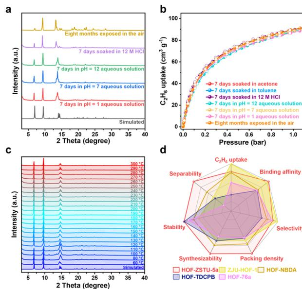
Fig. 6 (a) PXRD and (b)  $C_2H_6$  sorption isotherms of HOF-ZSTU-5a after undergoing several different environmental stability experiments. (c) Variable-temperature PXRD curve of HOF-ZSTU-5a. (d) A comprehensive comparison of  $C_2H_6$  uptake, binding affinity, selectivity, packing density, separability, stability, and synthesizability of HOF-ZSTU-5a and other high-performance carboxylic acid-based HOFs.
