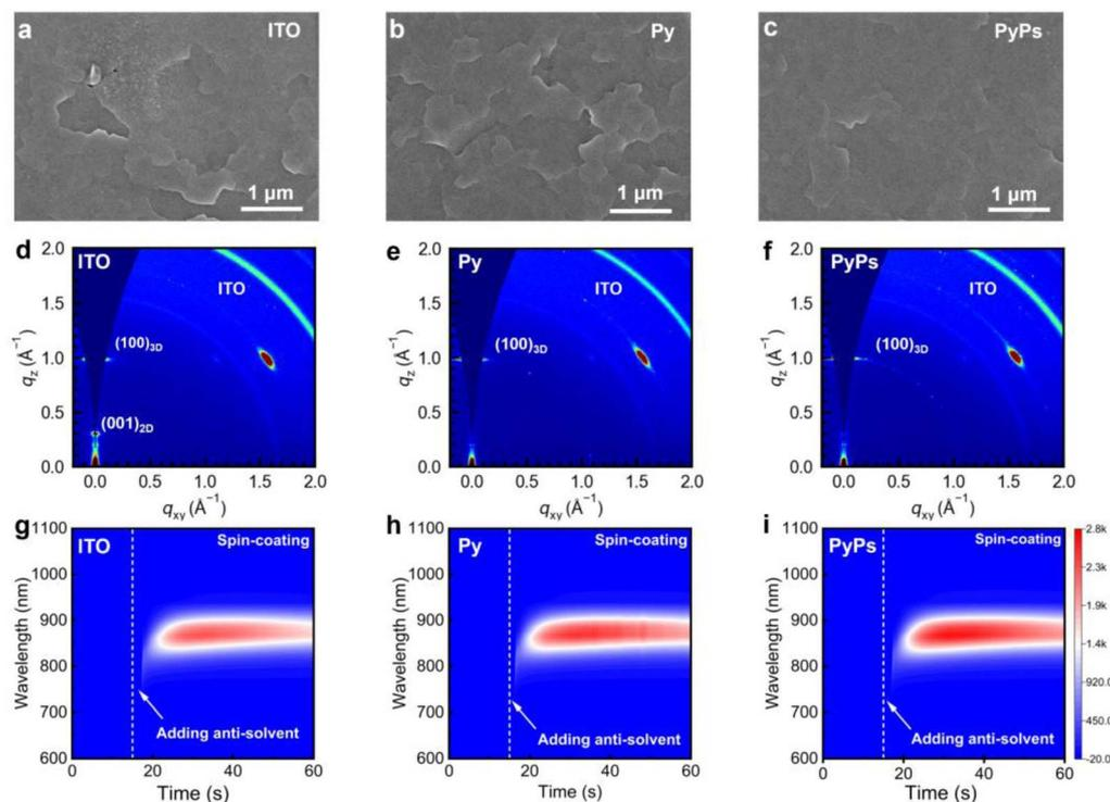
Fig. 2 Effects of HSLs on perovskite crystallinity. (a–c) Top-view SEM images of perovskite films on ITO, Py and PyPs substrates, respectively. (d–f) GIWAXS patterns of the perovskite films on ITO, Py and PyPs substrates, respectively. (g–i) *In situ* PL spectra of perovskite films deposited on different substrates.
