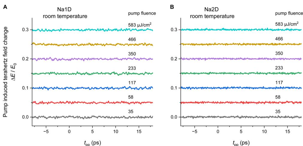
Fig. 5 400 nm optical pump terahertz transmission probe spectroscopy of **Na1D** (A) and **Na2D** (B) at 297 K. The pump-induced change of the transmitted terahertz electric field  $\Delta E/E_0$  is measured as a function of pump–probe time delay  $t_{\text{pp}}$  for various fluences of the 400 nm pump pulses, where  $E_0$  denotes the peak electric field of the terahertz probe pulse without the optical pump.
