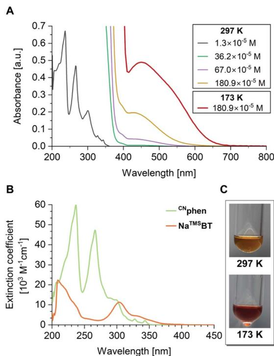
Fig. 6 (A) Concentration-dependent absorption spectra recorded upon dissolving **Na1D** in THF. (B) Absorption spectra of  $\text{CN}^{\text{phen}}$  (green) and  $\text{Na}^{\text{TMS}^{\text{BT}}}$  (orange) in THF solution. (C) Photographs of solutions of **Na1D** ( $\sim 180 \times 10^{-5}$  M) at 297 K (top) and 173 K (bottom).
