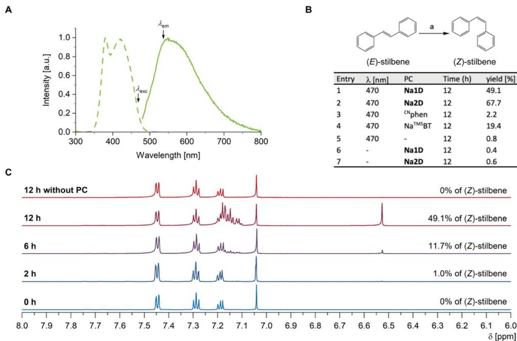
Fig. 7 Solution luminescence and energy transfer. (A) Luminescence (solid) and excitation (dashed) spectra of **Na1D** in THF ( $\lambda_{ex}$  = 470 nm,  $\lambda_{em}$  = 525 nm). (B) Photoisomerization of (*E*)-stilbene, a = photocatalytic conditions are summarized in the table. (C) Example of the low-field part of <sup>1</sup>H NMR spectra showing photocatalytic conversion of (*E*)-stilbene to (*Z*)-stilbene using **Na1D** solution and 470 nm irradiation.
