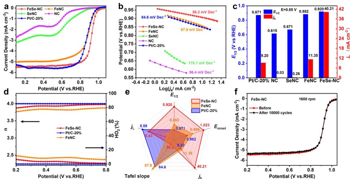
Fig. 4 Electrocatalytic ORR performance of FeSe-NC. (a) LSV polarization curves, (b) Tafel plots, and (c)  $E_{1/2}$  and  $j_k$  of FeSe-NC, FeNC, SeNC, NC, and Pt/C-20%. (d)  $\text{H}_2\text{O}_2$  yield (%) and electron transfer number ( $n$ ) obtained from RRDE tests of FeSe-NC, FeNC, and Pt/C-20%. (e) Performance radar chart of  $E_{\text{onset}}$ ,  $E_{1/2}$ , Tafel slope,  $j_k$  and  $j_L$  of FeSe-NC, FeNC and Pt/C-20%. (f) Accelerated degradation tests for the ORR of FeSe-NC.
