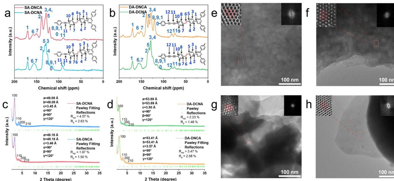
Fig. 1 (a and b)  $^{13}\text{C}$  ssNMR spectra of SA-DCNA and SA-DNCA, and DA-DCNA and DA-DNCA. (c and d) Experimental and simulated PXRD patterns of SA-DCNA and SA-DNCA, and DA-DCNA and DA-DNCA. (e–h) TEM images of SA-DCNA, SA-DNCA, DA-DCNA, and DA-DNCA. Left inset: enlarged image of the region within the red dotted box. Right inset: corresponding SAED pattern of the region within the red dotted box.
