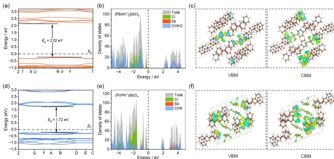
Fig. 4 (a) and (d) Calculated band structures, (b) and (e) density of states (DOS), and (c) and (f) electron density distributions of VBM and CBM of (a)–(c) (PBAH<sup>+</sup>)<sub>2</sub>SbCl<sub>5</sub> and (d)–(f) (PVPH<sup>+</sup>)SbCl<sub>4</sub>.
