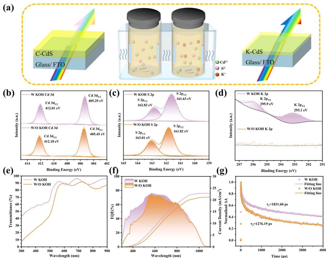
Fig. 1 (a) Schematic illustration of the CdS thin film deposition via chemical bath method, highlighting the structural differences between undoped (C-CdS) and K<sup>+</sup>-doped (K-CdS) samples, along with their respective short-wavelength light transmittance characteristics. (b–d) XPS spectra of Cd 3d, S 2p, and K 2p. (e) the transmission spectra, (f) EQE plot, (g) carrier decay curves extracted from TAS.
