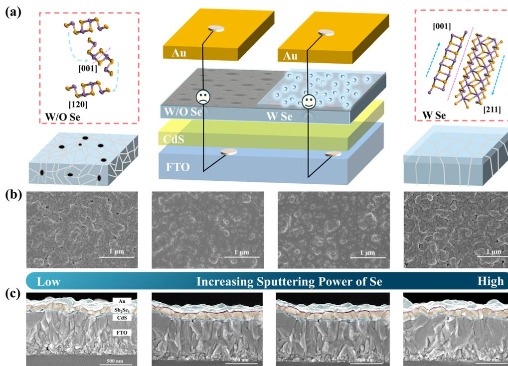
Fig. 2 (a) Schematic illustration of the  $Sb_2Se_3$  device structure, comparing the layer configuration, crystal orientation, and vertical carrier transport pathways under conditions W/O Se and W Se compensation. (b) and (c) The surface and cross-sectional SEM images of  $Sb_2Se_3$  films with Se interface layers deposited under different sputtering powers (0W, 18W, 22W, 26W).
