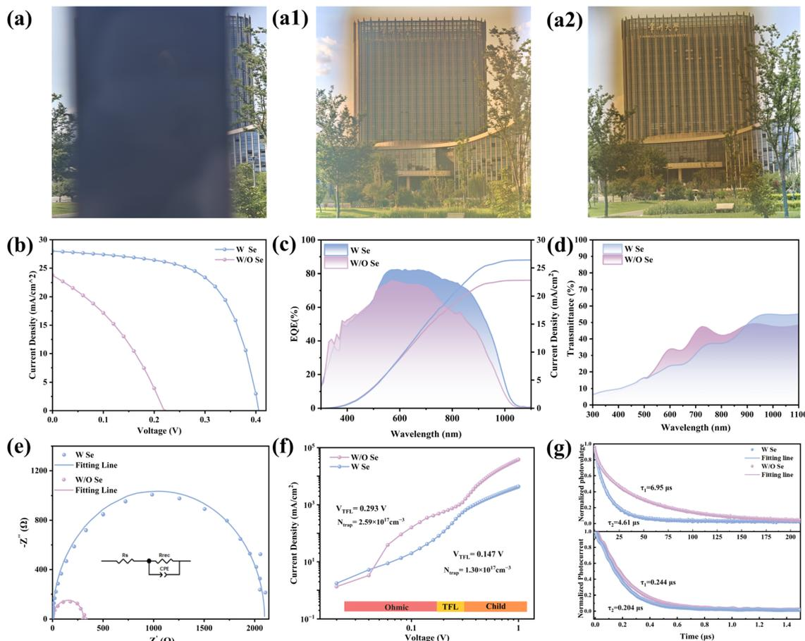
Fig. 5 Comparison of the semi-transparent appearance of (a) a 500 nm-thick  $\text{Sb}_2\text{Se}_3$  film, (a1) an ultrathin 50 nm W/O Se film, and (a2) a W Se film treated with active Se. (b)  $J$ - $V$  curves. (c) EQE plot, (d) transmission spectra, (e) Nyquist plots, (f) SCLC curves, (g) TPC and TPV decay curves of the corresponding  $\text{Sb}_2\text{Se}_3$  solar cells.
