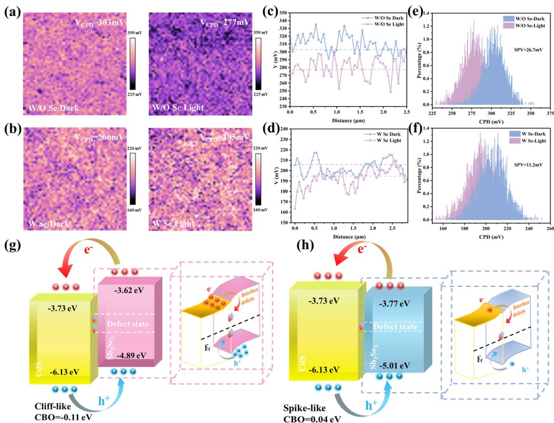
Fig. 4 (a and b) The KPFM (CPD) for the  $\text{Sb}_2\text{Se}_3$  samples W/O and W Se; (c and d) corresponding surface potential line profiles; (e and f) statistical distribution histograms of surface potential for both samples; schematic energy band structures of the CdS/ $\text{Sb}_2\text{Se}_3$  heterojunction W/O Se compensation (g) and W Se compensation (h).
