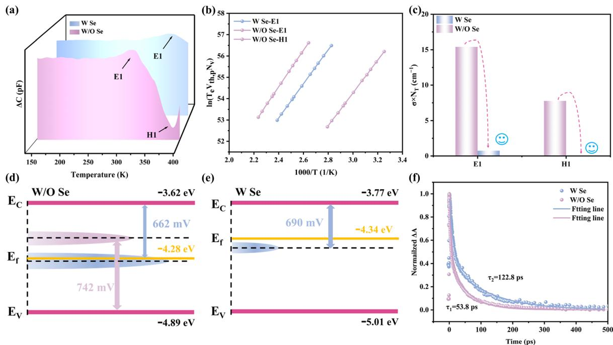
Fig. 6 (a) The capacitance variation of W/O Se and W Se samples at different temperatures. (b) Arrhenius plots; (c) comparison of  $\sigma \times N_T$  values; (d and e) defect energy level diagrams of the  $\text{Sb}_2\text{Se}_3$  solar cells with and without Se; (f) carrier lifetime of the  $\text{Sb}_2\text{Se}_3$  solar cells with and without Se.
