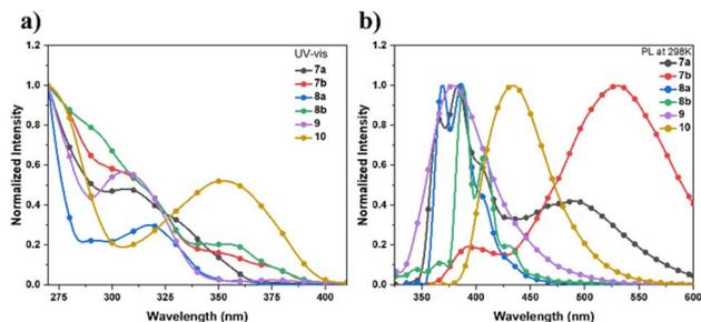
Fig. 1 (a) Absorption spectra and (b) fluorescence emission spectra of **7a**, **7b**, **8a**, **8b**, **9**, and **10** in  $\text{CH}_2\text{Cl}_2$  ( $1.0 \times 10^{-5}$  M).
