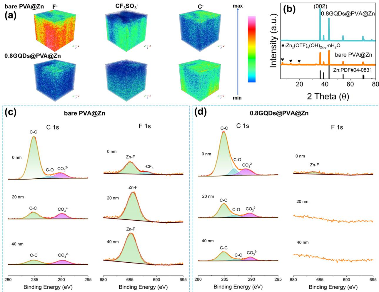
Fig. 4 Comparison of SEI composition and distribution on the zinc anode surface using different hydrogel electrolytes. (a) 3D visualization of TOM-SIMS depicting F<sup>-</sup>, CF<sub>3</sub>SO<sub>3</sub><sup>-</sup> and C<sup>-</sup> signals. (b) XRD patterns after cycling tests at 1 mA cm<sup>-2</sup>. XPS depth profile for C 1s and F 1s of the Zn anode surface with bare PVA@Zn (c) and 0.8GQDs@PVA@Zn (d).
