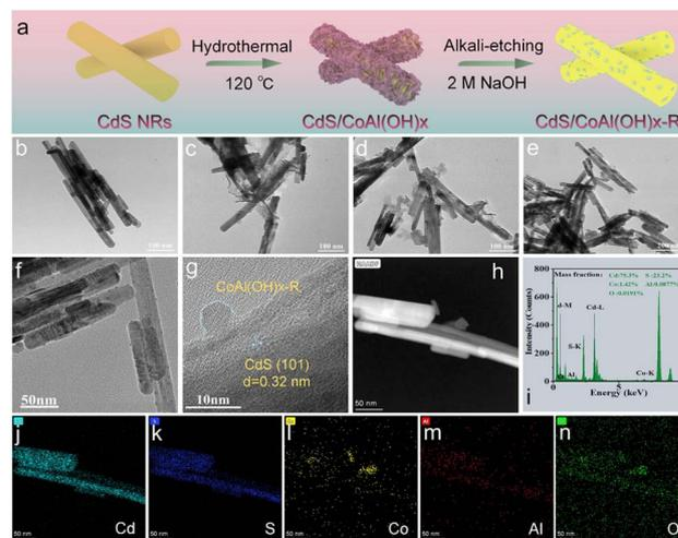
Fig. 1 (a) Schematic diagram of the preparation process, TEM image of (b) CdS, (c) CdS/Co(OH)<sub>x</sub>, (d) CdS/CoAl(OH)<sub>x</sub>, and (e and f) CdS/CoAl(OH)<sub>x</sub>-R, (g) HR-TEM images of CdS/CoAl(OH)<sub>x</sub>-R and (h–n) the corresponding elemental mapping.
