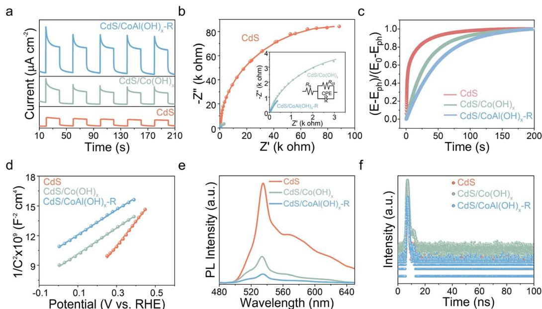
Fig. 5 (a) Transient photocurrent response, (b) EIS curves, (c) open-circuit potential decay curves, (d) M-S curves, (e) PL spectra, (f) TRPL spectra of CdS, CdS/Co(OH)<sub>x</sub> and CdS/CoAl(OH)<sub>x</sub>-R.
