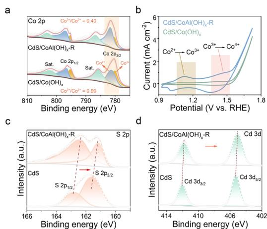
Fig. 4 High-resolution XPS spectra of (a) Co 2p, (b) CV curves for CdS, CdS/Co(OH)<sub>x</sub> and CdS/CoAl(OH)<sub>x</sub>-R, and (c) high-resolution XPS spectra of S 2p and (d) Cd 3d.
