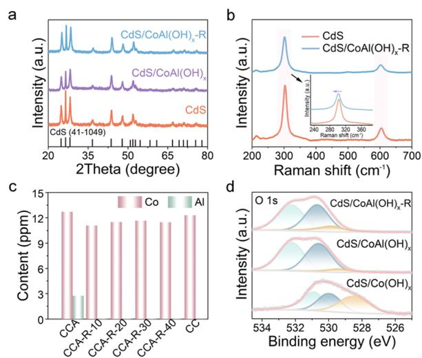
Fig. 2 (a) XRD patterns of the as-prepared samples, (b) Raman spectra of CdS and CdS/CoAl(OH)<sub>x</sub>-R, (c) ICP-OES results of elements in CdS/CoAl(OH)<sub>x</sub>-R with different alkali etching time. CCA: CdS/CoAl(OH)<sub>x</sub>, CCA-R-10: CdS/CoAl(OH)<sub>x</sub>-R-10 min, CCA-R-20: CdS/CoAl(OH)<sub>x</sub>-R-20 min, CCA-R-30: CdS/CoAl(OH)<sub>x</sub>-R-30 min, CCA-R-40: CdS/CoAl(OH)<sub>x</sub>-R-40 min, and CC: CdS/Co(OH)<sub>x</sub>, (d) high resolution XPS spectra of O 1s.
