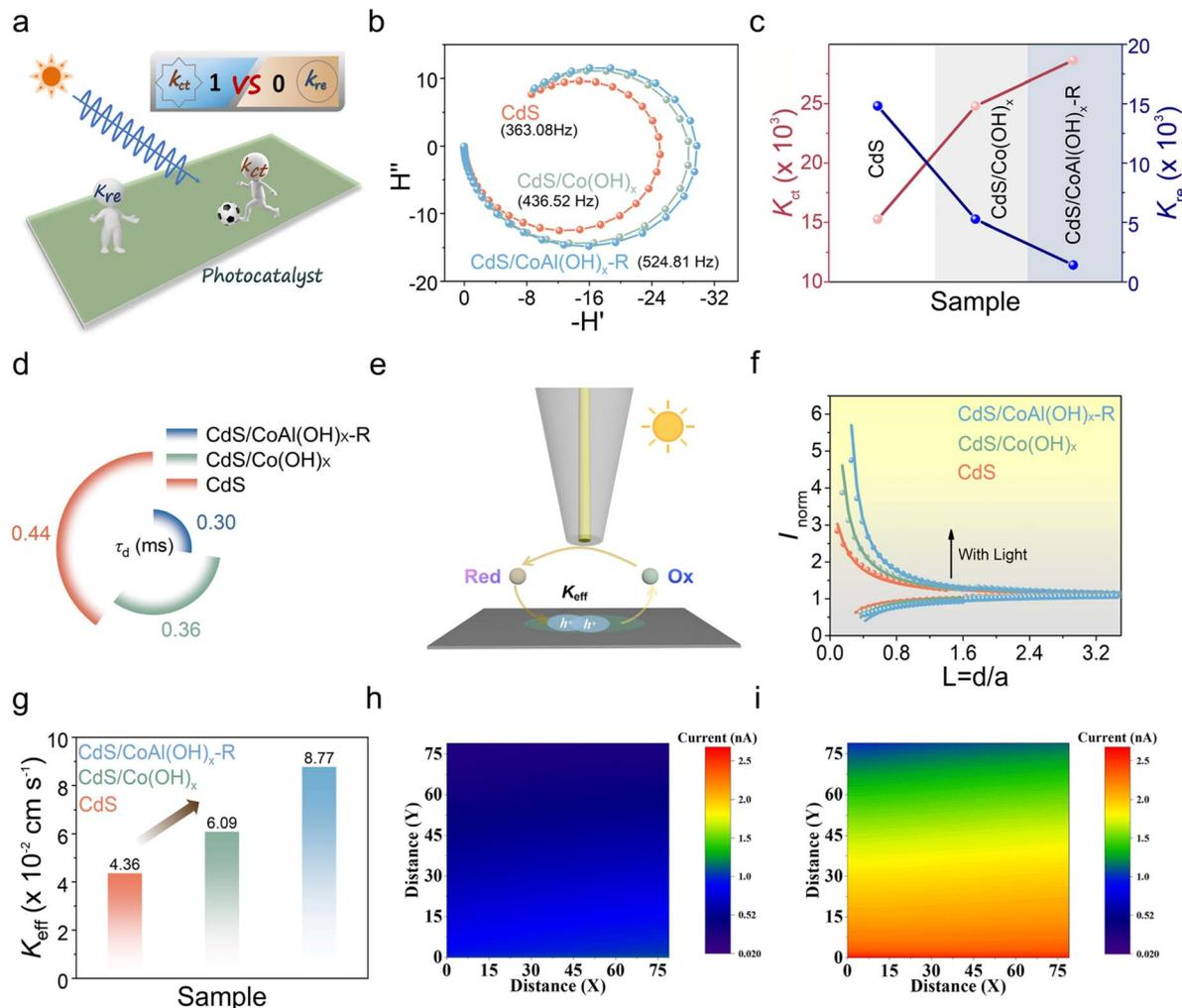
Fig. 6 (a) Principle of the IMPS setup, (b) IMPS curves, (c)  $K_{re}$  and  $K_{ct}$  values of CdS, CdS/Co(OH)<sub>x</sub> and CdS/CoAl(OH)<sub>x</sub>-R, (d)  $\tau_d$  values, (e) principle of the SPECM setup, (f) probe approach curves, (g)  $K_{eff}$  of CdS, CdS/Co(OH)<sub>x</sub> and CdS/CoAl(OH)<sub>x</sub>-R, (h) and (i) SPECM images of the CdS/CoAl(OH)<sub>x</sub>-R surface under dark and light conditions.
