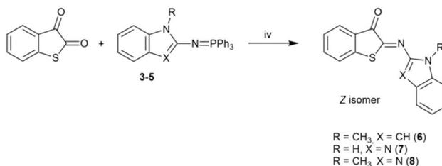
Scheme 1 Synthesis of HA-ITI photoswitches 6–8. Reagents and reaction conditions: (i) TsN<sub>3</sub>, *n*-BuLi, Et<sub>2</sub>O, reflux, 70% yield; (ii) PPh<sub>3</sub>, Et<sub>2</sub>O, 0 °C, 30% yield; (iii) Ph<sub>3</sub>PBr<sub>2</sub>, toluene, Et<sub>3</sub>N, reflux, 72–80% yield; (iv) toluene, 90 °C, overnight, 15–65% yield.
