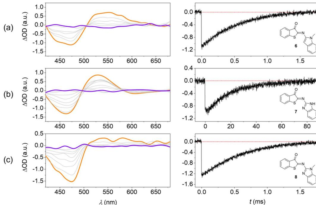
Fig. 5 Transient absorption spectroscopy confirms fast thermal  $E \rightarrow Z$  isomerization of HA-ITI photoswitches at room temperature. (Left) Transient absorption spectra of (a) **6**, (b) **7**, and (c) **8** in MTHF at room temperature; excitation at 355 nm, orange: spectrum after laser flash, purple: spectrum after complete ground-state recovery. (Right) Recovery kinetics of the  $Z$  form at 460 nm.
