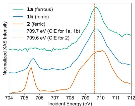
Fig. 3 Total electron yield Fe L<sub>3</sub>-edge XAS spectra with vertical lines showing energies where constant incident energy RIXS spectra were fit.
