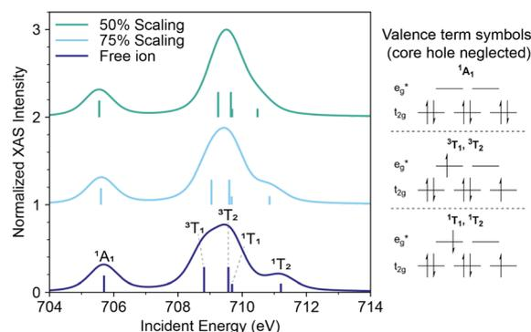
Fig. 4 Iron L<sub>3</sub>-edge XAS simulations for a  $d^5$  ground state (term symbols are for the  $d^6$  final states, which are schematically represented on the right). A 10 Dq of 4.3 eV was used for all plots, and the intensity was normalized to the maximum value of the plot showing 50% scaling of the  $F_{dd}^k$  parameter.
