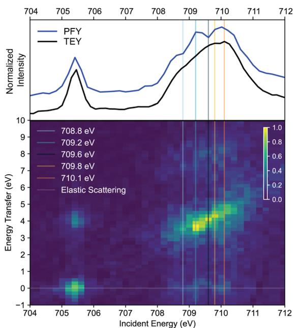
Fig. 5 Maximum-intensity-normalized 2D RIXS map of ferric complex **2** at the  $L_3$  absorption edge. PFY = partial fluorescence yield spectrum from integrated RIXS map. TEY = total electron yield spectrum from XAS. The vertical lines in the 709 to 710 eV area show the energies where CIE RIXS spectra were measured and averaged.
