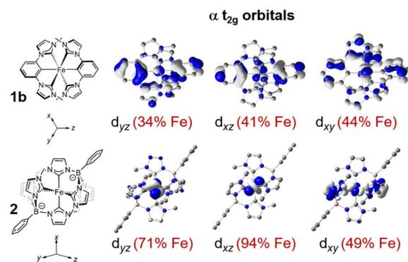
**Fig. 7** Comparison of DFT-derived  $t_{2g}$  orbital makeup of ferric **1b** and **2**, showing increased covalency for **1b** compared to **2**. The full orbital diagrams are shown in Fig. S10 and S11.
