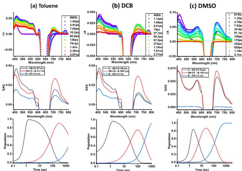
Fig. 6 Fs-TA absorption spectra at the indicated delay times of dimer **2** after exciting at 650 nm in (a) toluene, (b) *o*-DCB, and (c) DMSO, along with SAS spectra (middle row) and population decay curves (bottom row) where A and B represent  $^1\text{BDP}^*-\text{BDP}$  and  $^3\text{BDP}^*-\text{BDP}$ .
