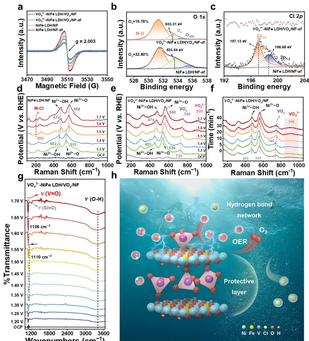
Fig. 3 Anti-corrosion property of  $\text{VO}_4^{3-}$ -NiFe LDH/ $\text{VO}_x$ /NF. (a) EPR spectra; (b and c) HRXPS spectra after stability testing; (d and e) potential-dependent Raman spectra; (f) time-dependent Raman spectra; (g) *In situ* FTIR spectra; (h) schematic diagram of the anti-corrosion mechanism.
