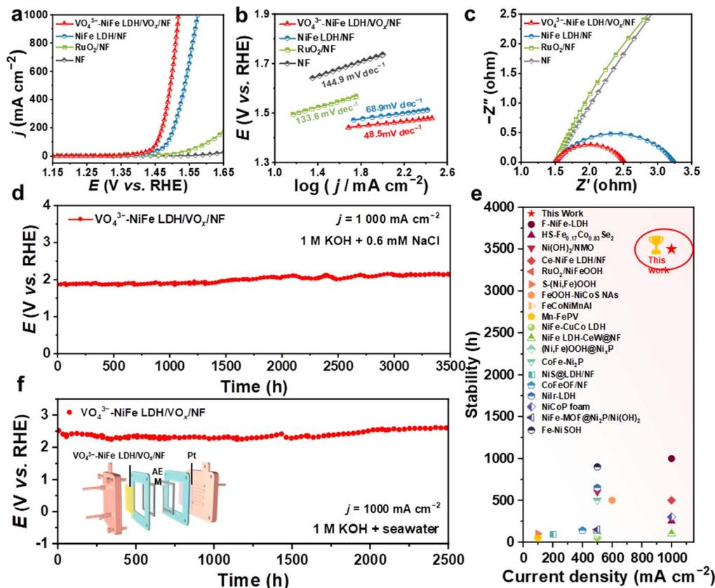
Fig. 2 (a) OER polarization curves of all catalysts in 1.0 M KOH + 0.6 M NaCl; (b) Tafel plots; (c) EIS Scheme; (d) durability evaluation by the chronopotentiometry at  $1000 \text{ mA cm}^{-2}$ ; (e) comparison of stability with other works; (f) durability evaluation using electrolysis membrane electrode assembly.
