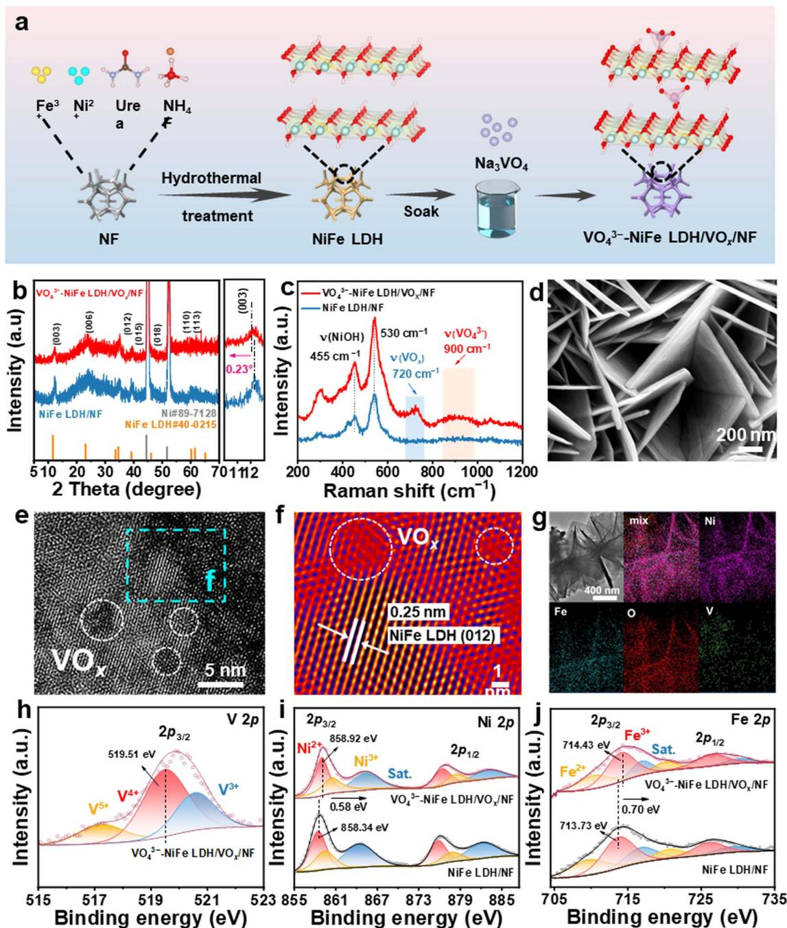
Fig. 1 Material characterization. (a) Schematic illustration of the synthesis process; (b) XRD patterns of  $\text{VO}_4^{3-}$ -NiFe LDH/ $\text{VO}_x$ /NF and NiFe LDH/NF; (c) Raman spectra; (d) SEM images of the  $\text{VO}_4^{3-}$ -NiFe LDH/ $\text{VO}_x$ /NF; (e) TEM picture; (f) HRTEM image; (g) TEM image and corresponding elemental distributions; (h–j) HRXPS spectra of V 2p, Ni 2p, and Fe 2p.
