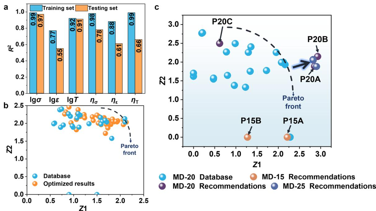
Fig. 3 Optimization results of the MD-25 models and all experimental results. (a) Single-objective model establishment:  $R^2$  values of MD-25. (b) The comprehensive performance index of mechanical and self-healing properties within the dataset, along with the Pareto front based on MD-25. (c) All experimental data in the  $Z_1$ - $Z_2$  plan.
